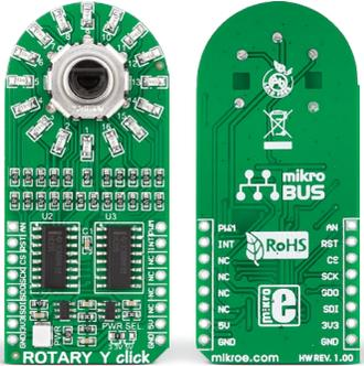
Rotary Y click carries a **15-pulse incremental rotary encoder** with detents, surrounded by a **ring of 16 yellow LEDs**. It communicates with the target board through mikroBUS™ **SPI lines** (CS, SCK, MISO, MOSI), and three additional lines for outputting the Encoder info: ENCB OUT, ENCA OUT and SW (in place of the standard AN, RST and INT pins, respectively). Rotary Y click can be used with either a 3.3V or 5V power supply.
