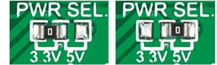
There is one zero-ohm SMD jumper J1 used to select whether 3.3V or 5V I/O voltage level is used. Jumper J1 is soldered in 3.3V position by default.
