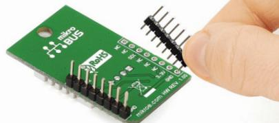
Turn the board upside down so that the bottom side is facing you upwards. Place shorter pins of the header into the appropriate soldering pads.
