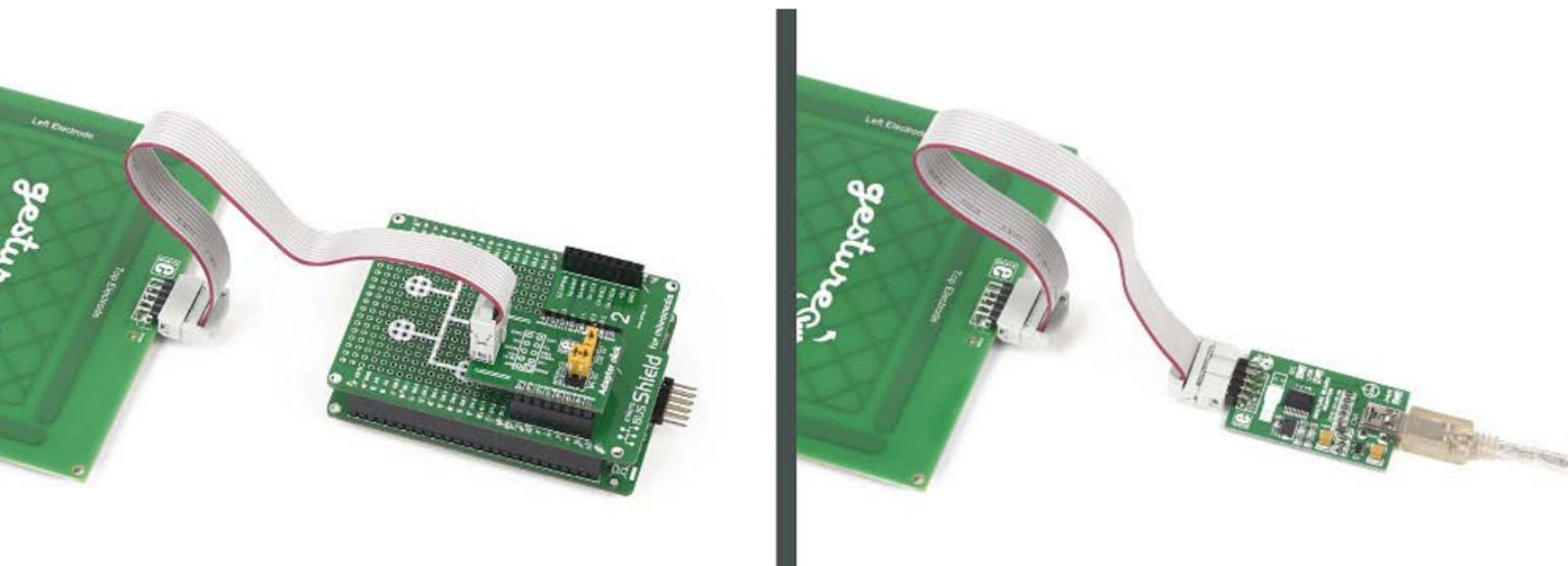
The Gesture board comes with an IDC10 connector cable. If you wish to use it for hardware prototyping, we suggest you pair it with adapter click. The other options is to develop PC applications. For that purpose we developed the Gesture USB adapter.
