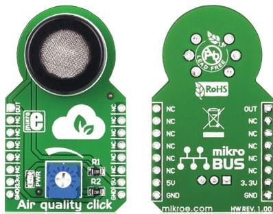
Air quality click™ is a simple solution for adding a high sensitivity sensor for detecting a variety of gases that impact air quality in homes and offices. The board features an MQ-135 sensor, a calibration potentiometer, a mikroBUS™ host socket, two jumpers and a power indicator LED. Air quality click™ communicates with the target board through mikroBUS™ AN (OUT) line. Air quality click™ is designed to use a 5V power supply only.
