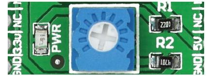
To calibrate Methane click™ for optimum performance, use the on-board potentiometer to adjust the load resistance of the sensor circuit.
