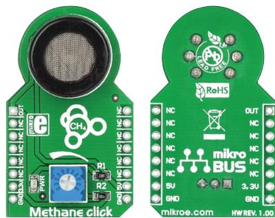
Methane click™ is a simple solution for adding a high sensitivity methane ( $\text{CH}_4$ ) sensor to your design. It's suitable for designing gas leakage equipment. The board features an MQ-4 sensor, a calibration potentiometer, a mikroBUS™ host socket, two jumpers and a power indicator LED. Methane click™ communicates with the target board through mikroBUS™ AN (OUT) line. Methane click™ is designed to use a 5V power supply only.
