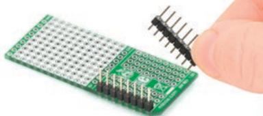
Turn the board upside down so that bottom side is facing you upwards. Place shorter pins of the header into the appropriate soldering pads.
