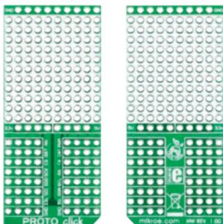
PROTO click™ is an accessory board in **mikroBUS™** form factor. It features 10x11 prototyping area as well as additional power pads. It can be used to assemble custom electronics thus creating a custom click™ board. PROTO click™ contains **mikroBUS™** I<sup>2</sup>C (SDA, SCL), SPI (MISO, MOSI, SCK, CS), UART (TX, RX), PWM, INT, AN and RST lines from the target board microcontroller. The board provides 3.3 V and 5 V power supply.
