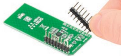
Turn the board upside down so that bottom side is facing you upwards. Place shorter pins of the header into the appropriate soldering pads.
