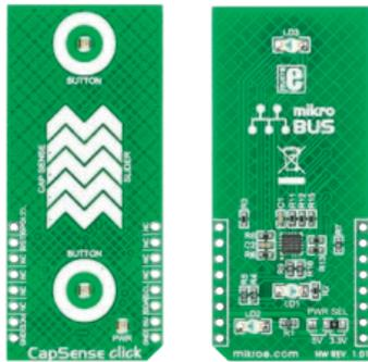
CapSense click™ is an accessory board in **mikroBUS™** form factor. It's a compact and easy solution for adding capacitive sensing elements to your design. It features **CY8C201A0** capacitive controller and capacitive sensing elements. CapSense click™ communicates with the target board microcontroller via **mikroBUS™** I<sup>2</sup>C (SDA, SCL), AN and RST lines. The board is designed to use 3.3 V or 5 V power supply. LED diode (GREEN) indicates the presence of power supply.
