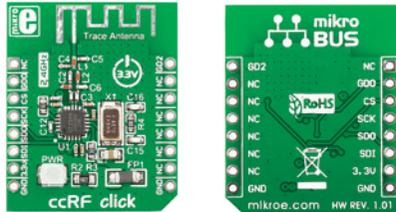
ccRF click™ is an accessory board in **mikroBUS™** form factor. It's a compact and easy solution for adding RF transceiver to your design. It features **CC2500** Low-Power 2.4 GHz RF transceiver as well as PCB trace antenna. ccRF click™ communicates with the target board microcontroller via **mikroBUS™** SPI (MOSI, MISO, SCK, CS), RST and PWM lines. The board is designed to use 3.3V power supply only. LED diode (GREEN) indicates the presence of power supply.
