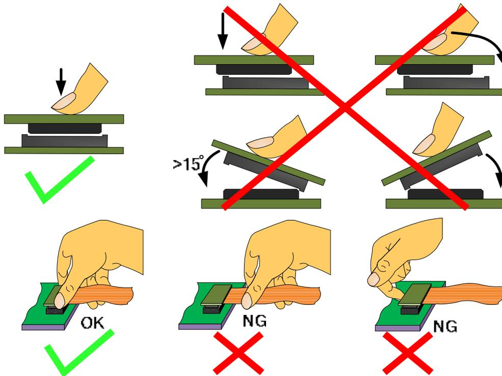
**Precaution for soldering the LCM**
