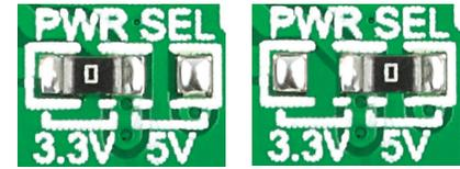
There is one zero-ohm SMD jumper **J1** used to select whether 3.3V or 5V power supply is used. Jumper **J1** is soldered in 3.3V position by default.
