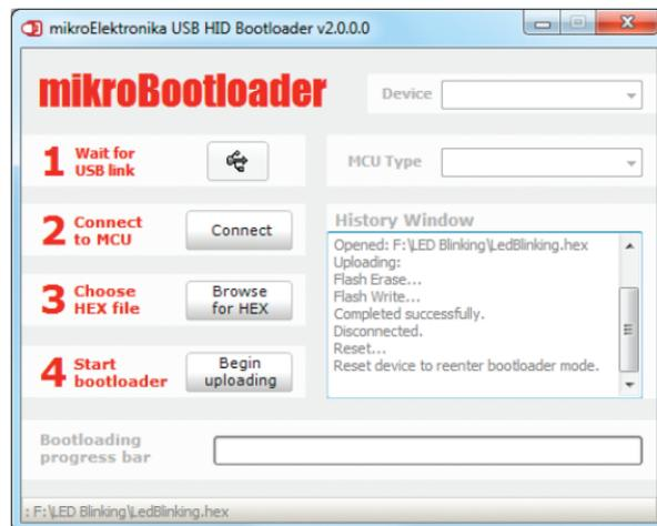
Figure 1-7: mikroBootloader ready for next job
