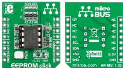
EEPROM Click™ is an accessory board in **mikroBUS™** form factor. It's a compact and easy solution for adding more EEPROM memory to your device. It features DIP **24C08** 8kbit serial EEPROM module in DIP 8 socket. EEPROM Click™ communicates with target board via I<sup>2</sup>C interface. The board is designed to use 3.3V and 5V power supply. It has a LED diode (GREEN) that indicates the presence of power supply.
