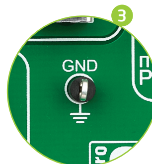
Figure 26-1: Three oscilloscope GND pins are conveniently positioned so different parts of the board can be reached with an oscilloscope probe
