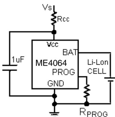
**Fig.3:A circuit to maximum the thermal regulation charge current  $V_{\text{CC}}$  bypass capacitor**
