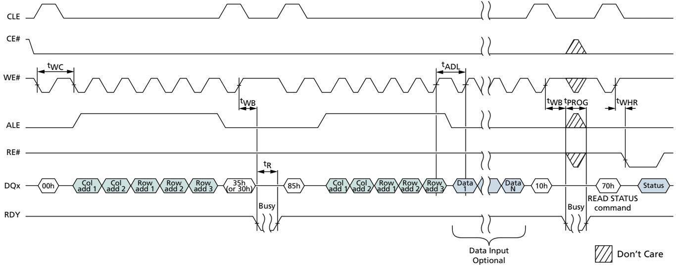
**Figure 68: ERASE BLOCK Operation**
