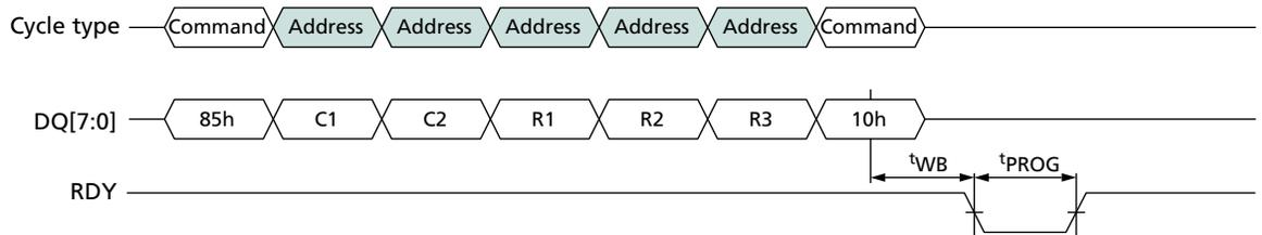
**Figure 44: COPYBACK PROGRAM (85h-10h) with CHANGE WRITE COLUMN (85h) Operation**
