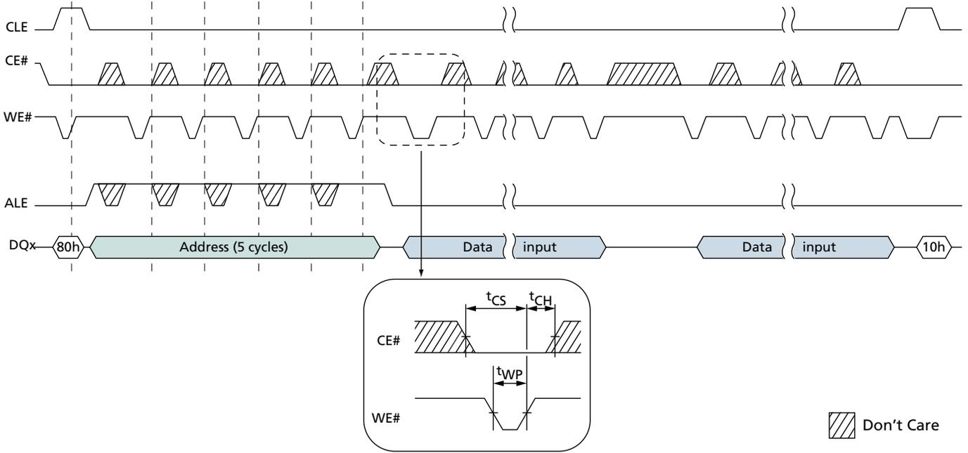
**Figure 64: PROGRAM PAGE Operation with CHANGE WRITE COLUMN**
