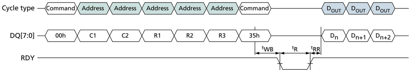
**Figure 42: COPYBACK READ (00h-35h) with CHANGE READ COLUMN (05h-E0h) Operation**
