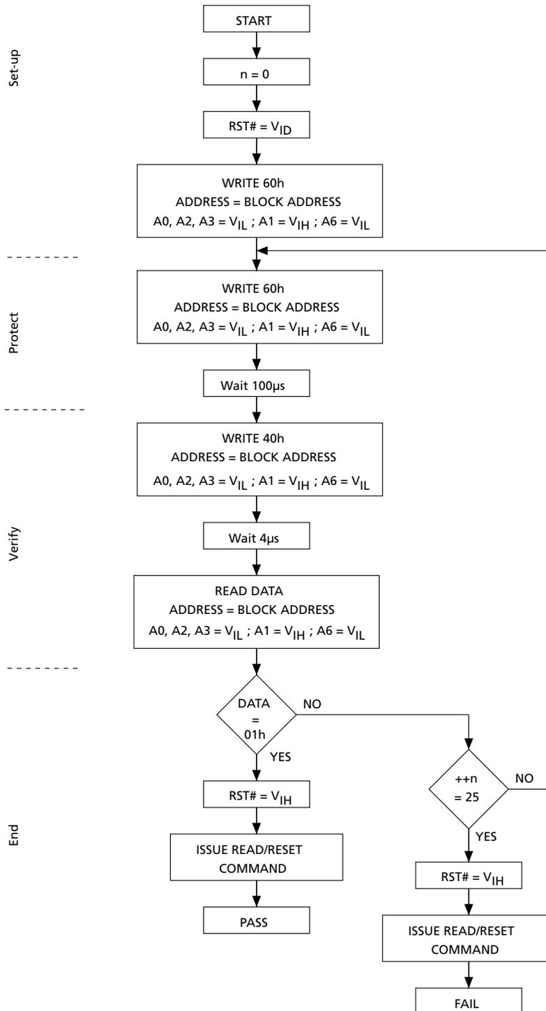
**Figure 9: In-System Equipment Chip Protect Flowchart**
