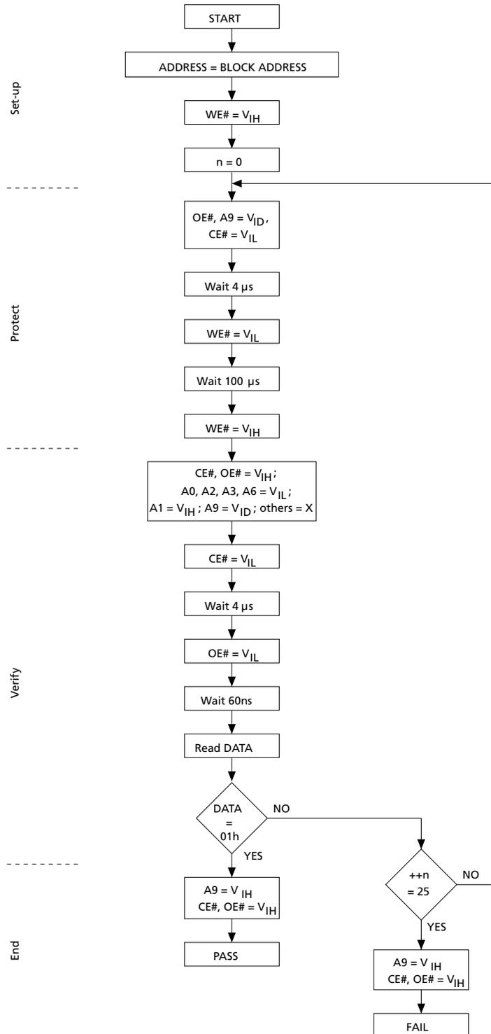
**Figure 7: Programmer Equipment Chip Unprotect Flowchart**
