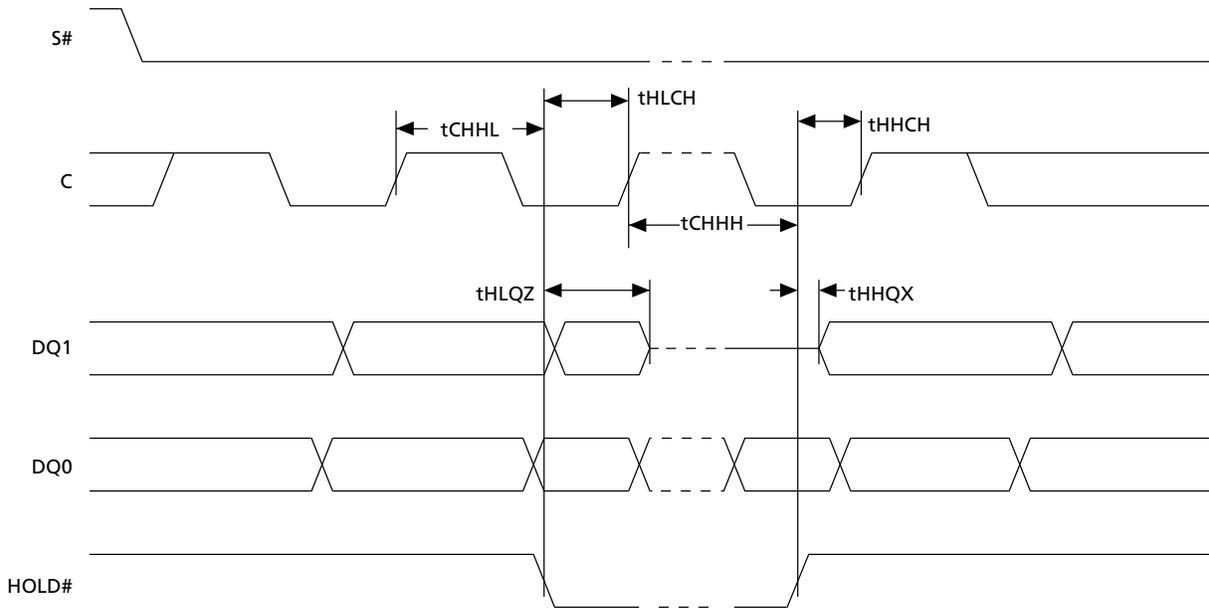
**Figure 27: Output Timing**
