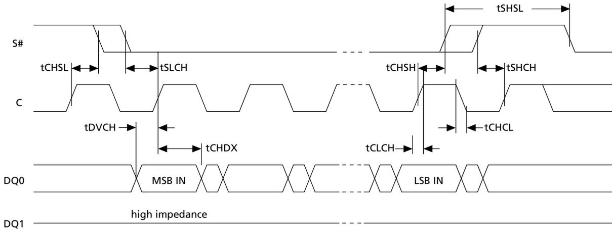
**Figure 25: Write Protect Setup and Hold During WRSR When SRWD=1 Timing**
