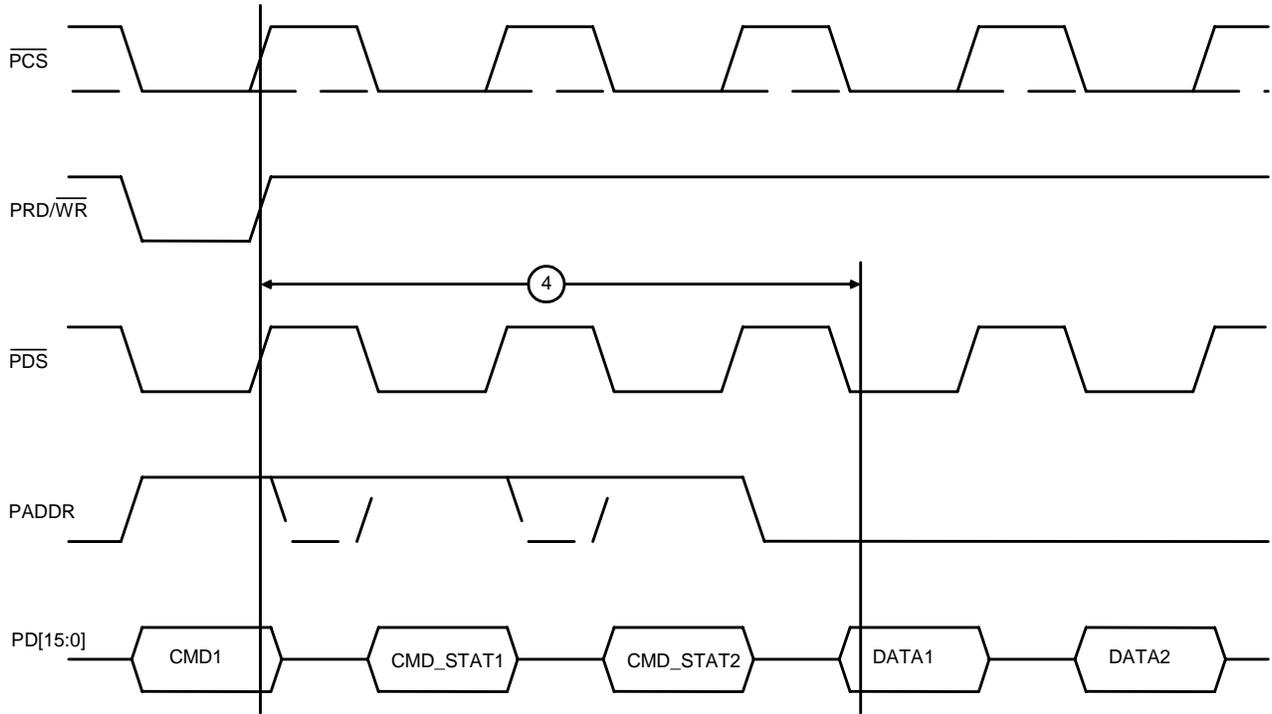
Note: Each Write and Read access is qualified by an active chip select strobe. (Chip select can be tied Low in some applications.)
