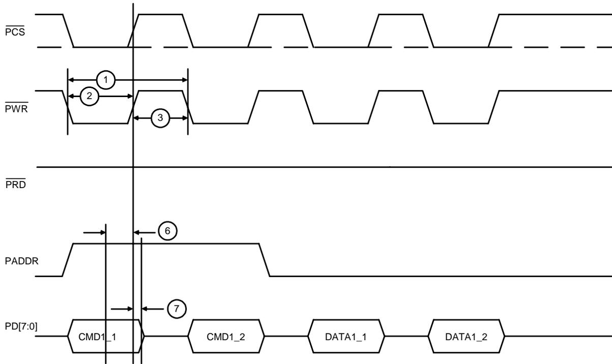
Note: Each Write and Read access is qualified by an active chip select strobe. (Chip select can be tied Low in some applications.)
