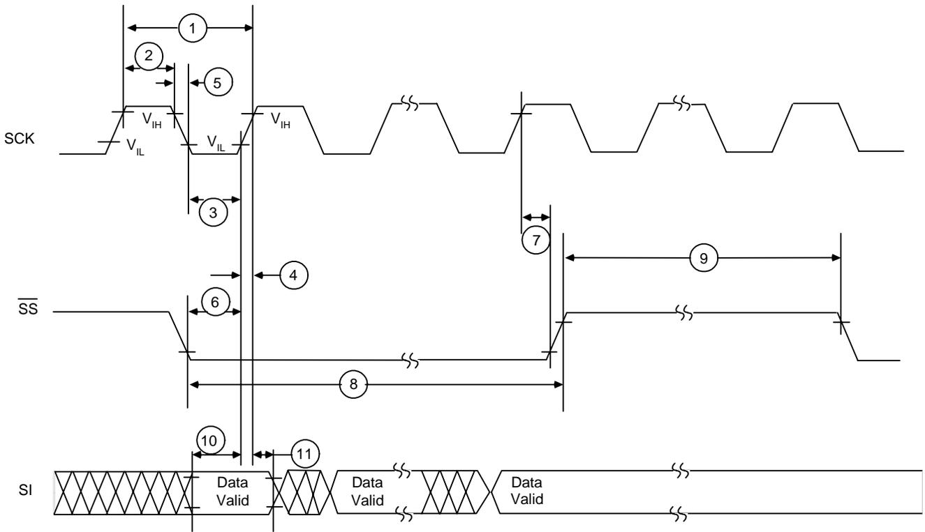
Figure 22. SPI Interface (Output Timing)
