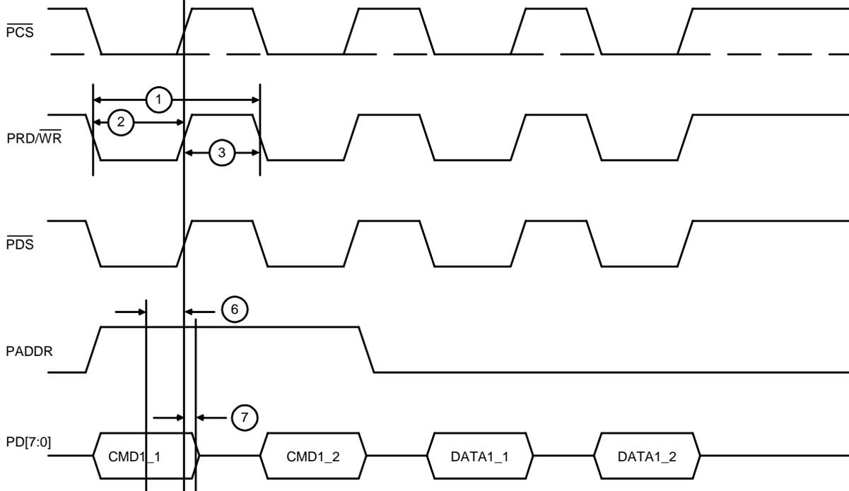
Note: Each Write and Read access is qualified by an active chip select strobe. (Chip select can be tied Low in some applications.)
