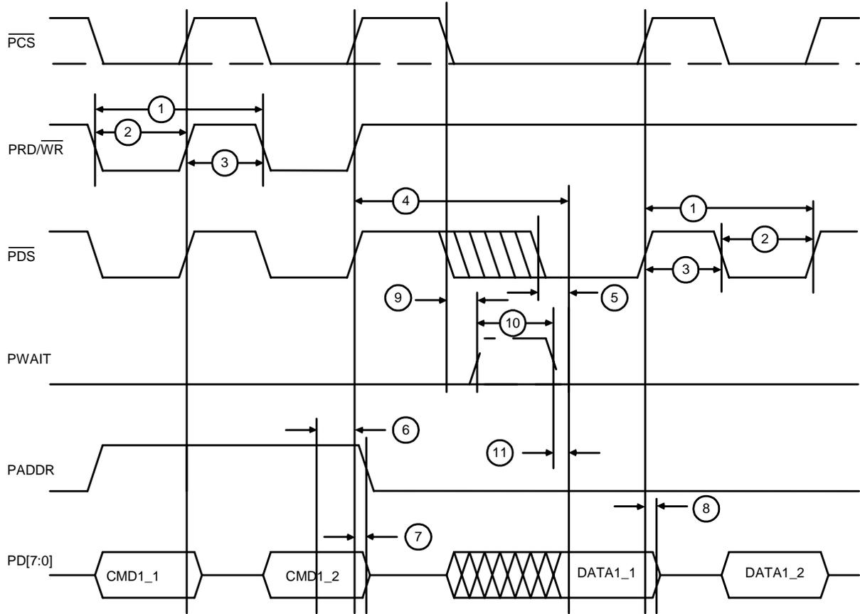
Note: Each Write and Read access is qualified by an active chip select strobe. (Chip select can be tied Low in some applications.)
