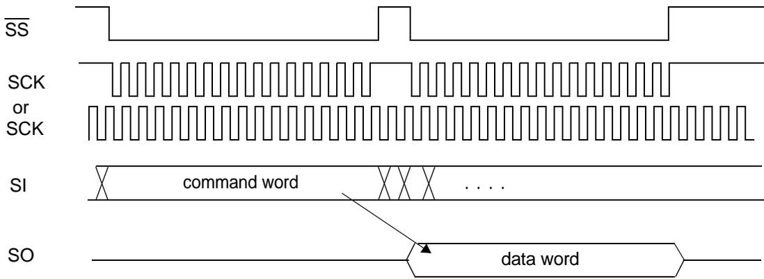
**Figure 20. One Data Word Write in Byte Framing Mode with Byte Swap**
