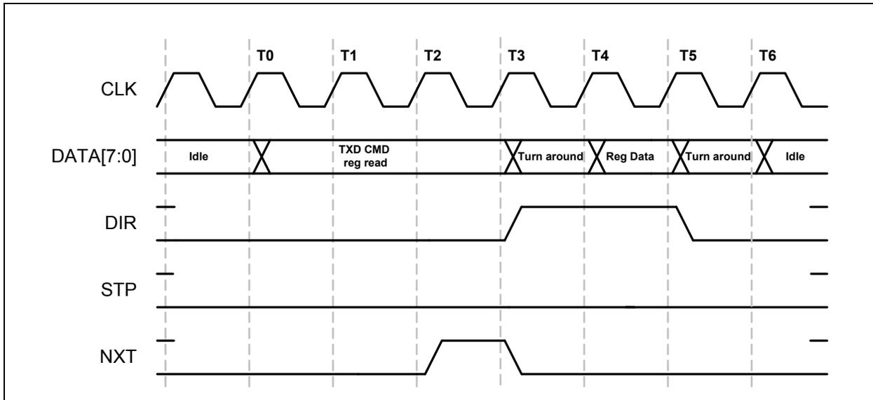
Figure 6.5 ULPI Register Read in Synchronous Mode
