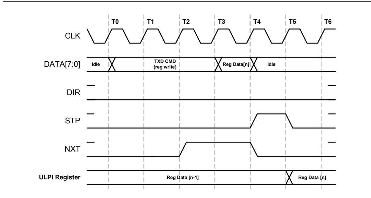
Figure 6.3 ULPI Register Write in Synchronous Mode
