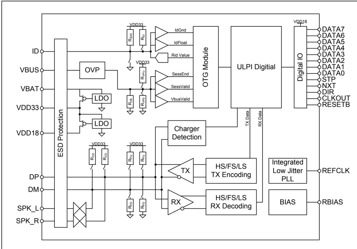
Figure 5.1 USB334x System Diagram (USB3341, USB3346, and USB3347)
