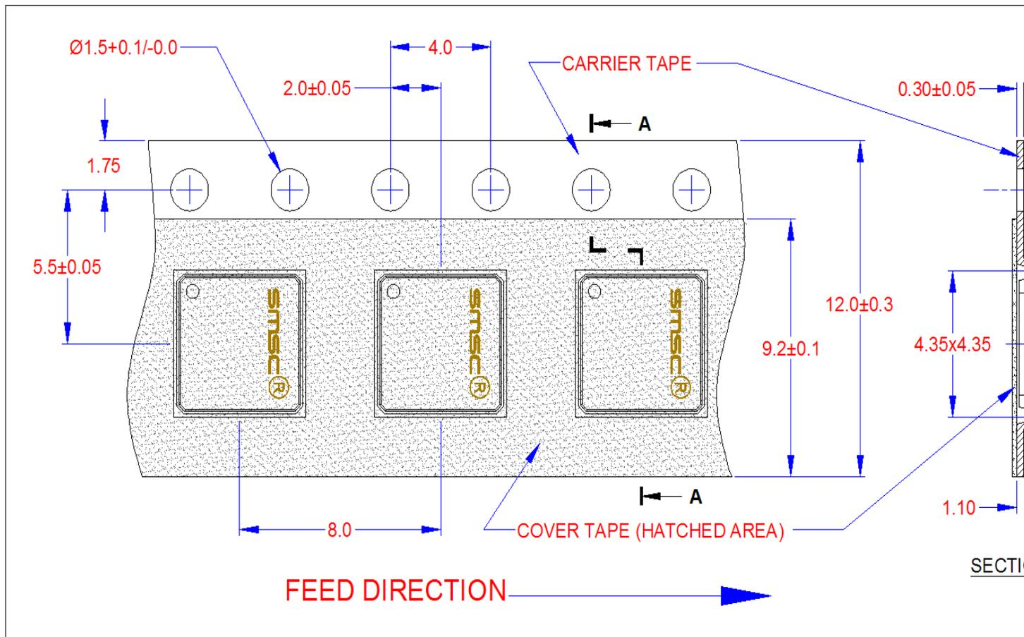
**QFN-4x4: TAPING DIMENSIONS AND PART ORIENTATION**
