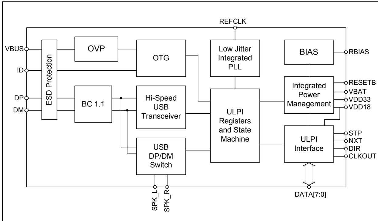
Figure 1.1 Block Diagram (USB3341, USB3346, and USB3347)
