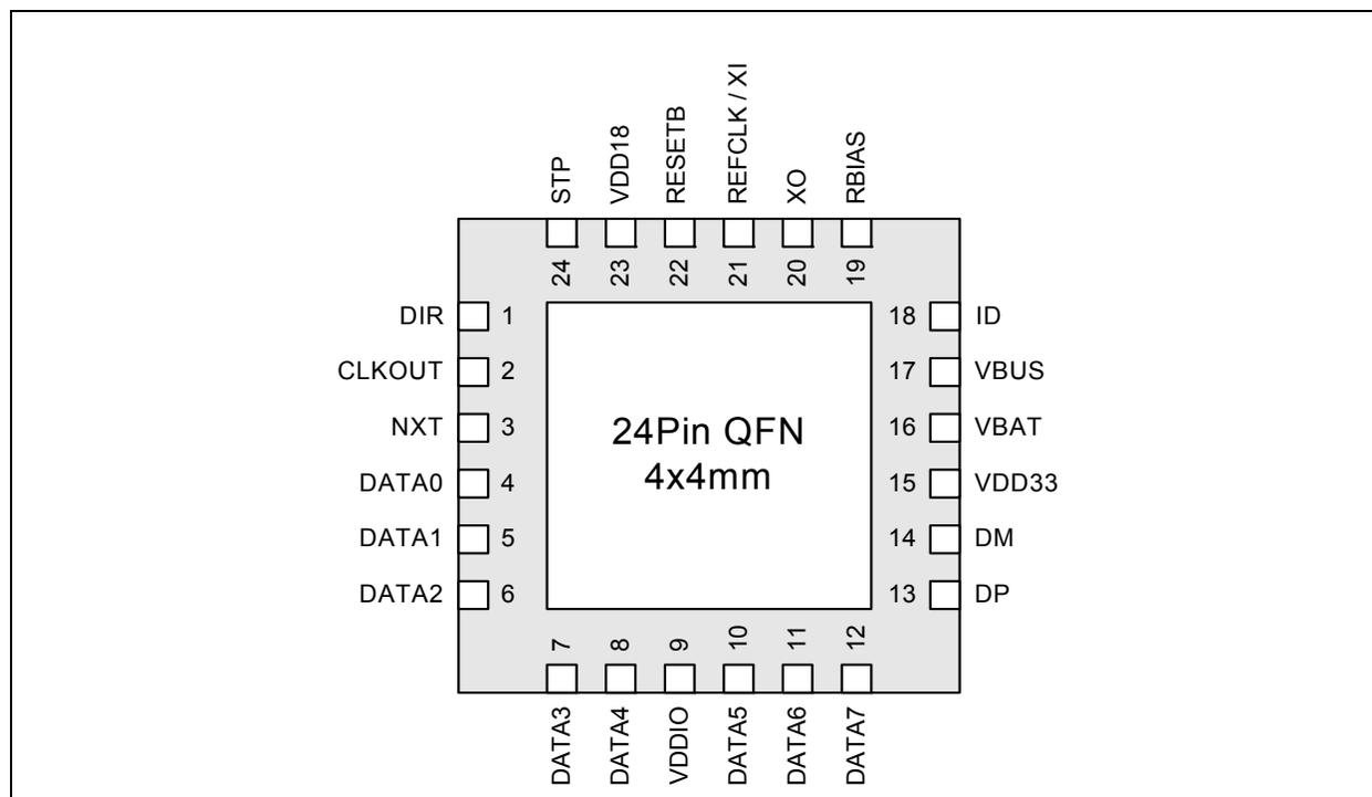
Figure 2.2 USB3343 Pin Locations - Top View
