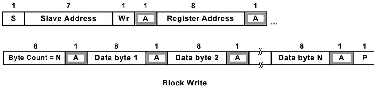
**Figure 4.1 Block Write**
