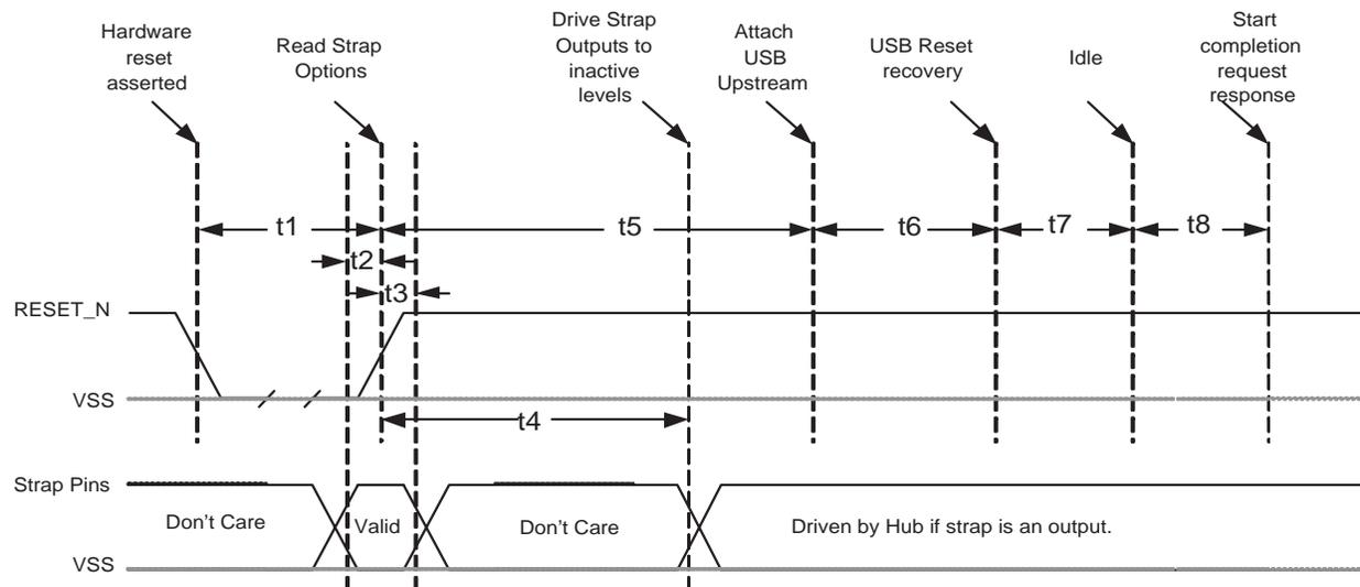
Figure 4.3 Reset\_N Timing for Default/Strap Option Mode
