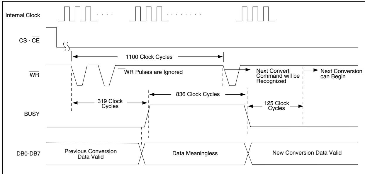
**FIGURE 8-5: BUS OUTPUT TIMING, DEMAND MODE**
