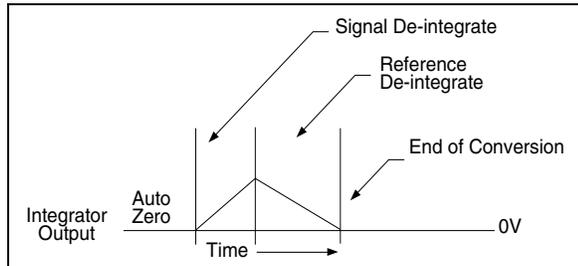
The input signal being converted is integrated for a fixed time period, measured by counting clock pulses. An opposite polarity constant reference voltage is then de-integrated until the integrator output voltage returns to zero. The reference integration time is directly proportional to the input signal.
