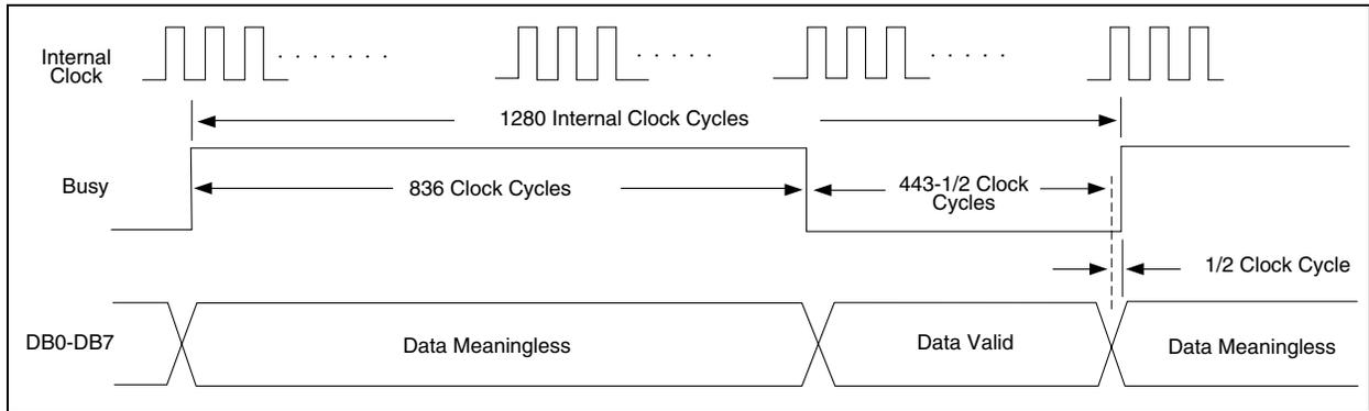
**FIGURE 8-7: BUS OUTPUT TIMING, CONTINUOUS MODE**
