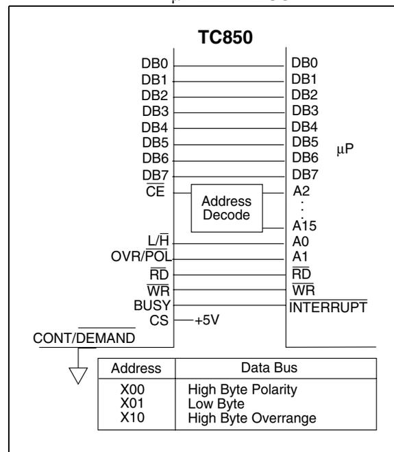
Figure 8-3 shows a typical interface to a  $\mu$ P I/O port or single-chip  $\mu$ C. The TC850 operates in the continuous mode and can either interrupt the  $\mu$ C/ $\mu$ P or be polled with an input pin.
