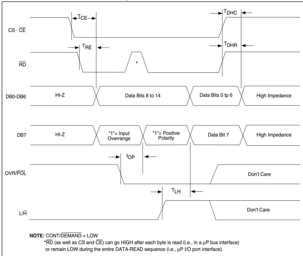
**FIGURE 8-6: CONVERSION TIMING, CONTINUOUS MODE**
