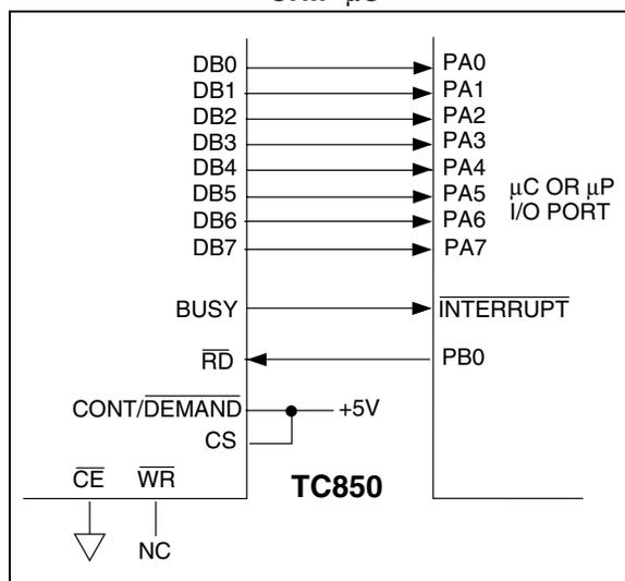
Since the PA0-PA7 inputs are dedicated to reading A/D data, the A/D CS/CE inputs can be enabled continuously. In continuous mode, data must be read in 3 bytes, as shown in Table 6-1. The required  $\overline{RD}$  pulses are provided by a  $\mu$ C/ $\mu$ P output pin.
