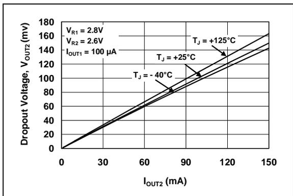
**FIGURE 2-8:** Dropout Voltage vs. Output Current ( $V_{OUT2}$ ).
