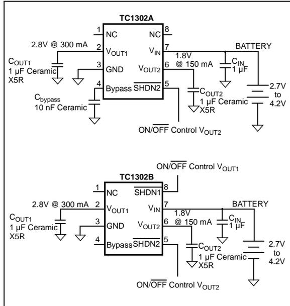
**FIGURE 6-1:** Typical Application Circuit TC1302A/B.
