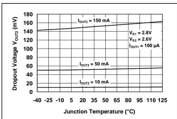
**FIGURE 2-9:** Dropout Voltage vs. Junction Temperature ( $V_{OUT2}$ ).
