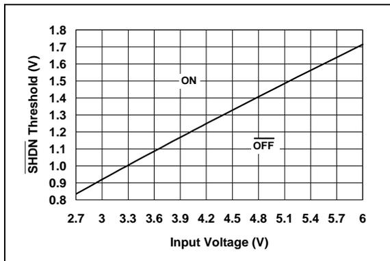
**FIGURE 2-2:**  $\overline{SHDN}$  Voltage Threshold vs. Input Voltage.
