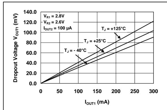
**FIGURE 2-6:** Dropout Voltage vs. Output Current ( $V_{OUT1}$ ).
