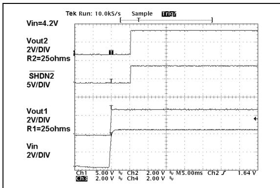
**FIGURE 2-21:**  $V_{OUT2}$  Power-up from Shutdown Input TC1302A.
