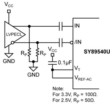
**Figure 5b. LVPECL Interface (AC-Coupled)**
