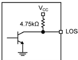
Figure 4. Input Structure
