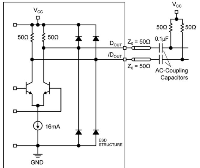
Figure 3. Output Structure
