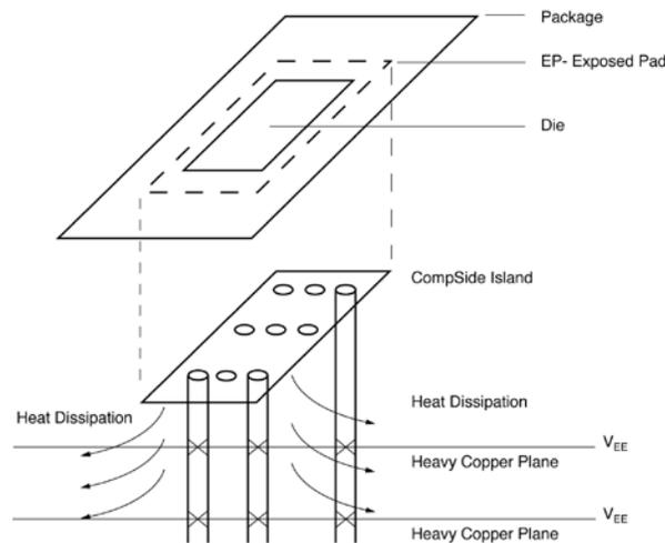
**PCB Thermal Consideration for 16-Pin QFN Package**
