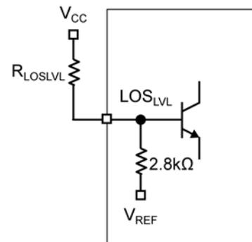
Figure 5. LOS<sub>LVL</sub> Setting Circuit
