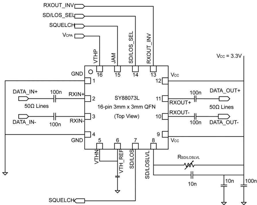
Note:  $V_{CPA}$  from DAC output or other voltage source.
