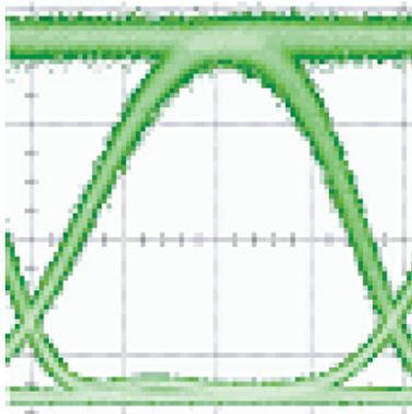
**Waveform 2: Minimum Crossing Point Adjustment (~30% Decision Threshold) – 20mV<sub>PP</sub> Signal Input**
