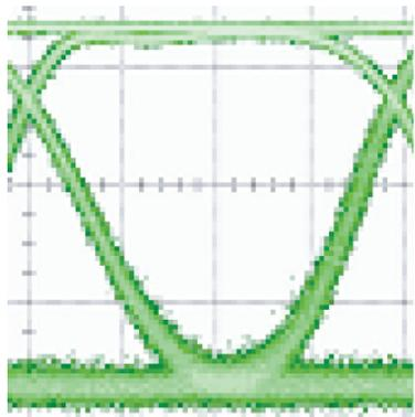
**Waveform 3: Minimum Crossing Point Adjustment (~70% Decision Threshold) – 20mV<sub>PP</sub> Signal Input**
