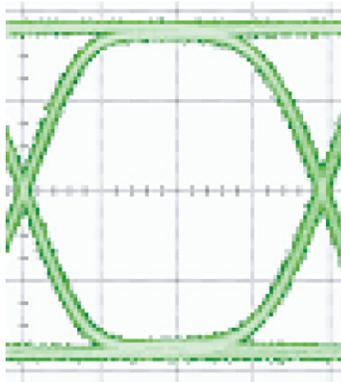
**Waveform 1: Nominal Crossing Point Adjustment (50% Decision Threshold) – 20mV<sub>PP</sub> Signal Input**
