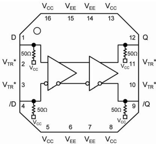
\*V<sub>TR</sub> is not connected to the DIE.
