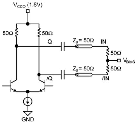
Figure 5c. CML AC-Coupled Termination
