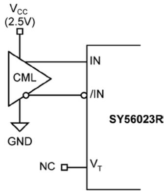
Figure 4a. CML Interface 100Ω Differential (DC-Coupled, 2.5V)
