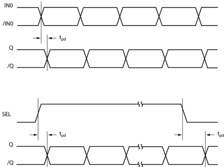
Figure 1. Propagation Delay
