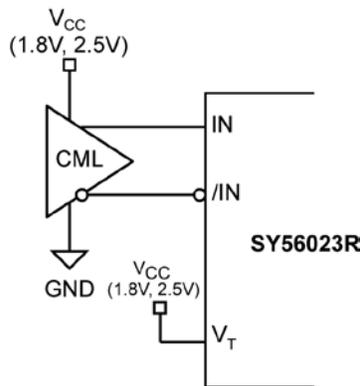
Figure 4b. CML Interface 50Ω to V<sub>CC</sub> (DC-Coupled, 1.8V, 2.5V)
