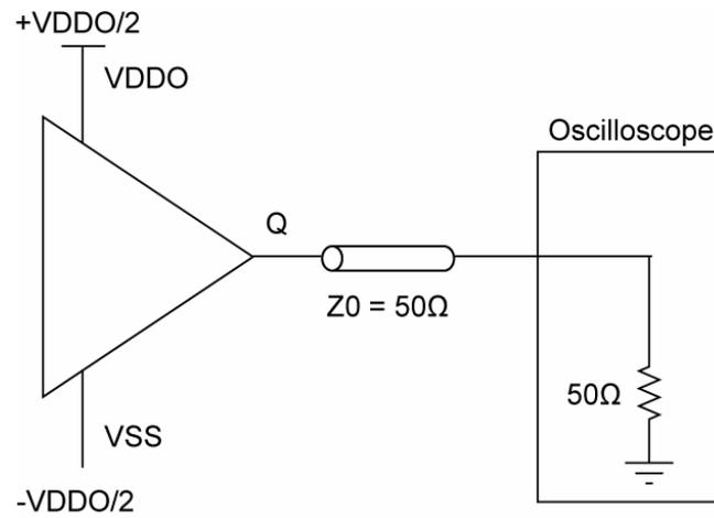
Figure 4. CMOS Output Load and Test Circuit
