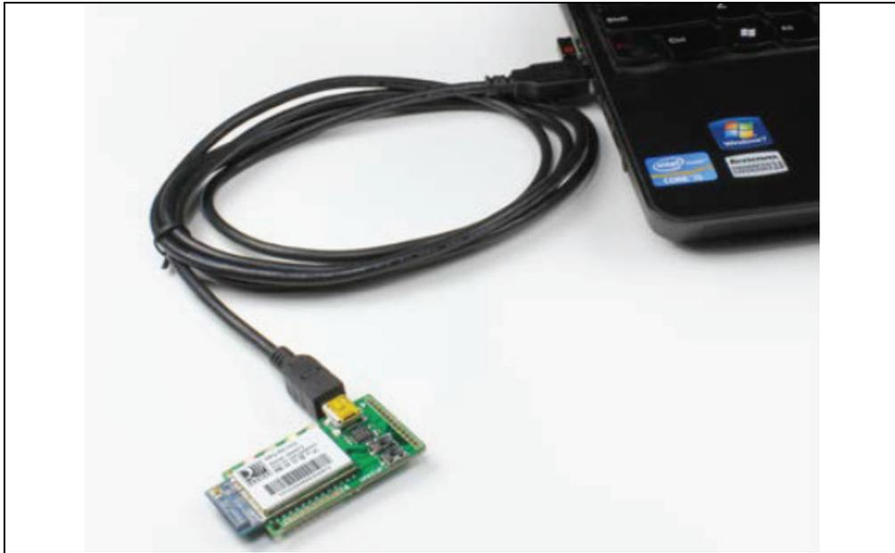
FIGURE 2-2: RN171 EVALUATION BOARD HARDWARE SETUP
