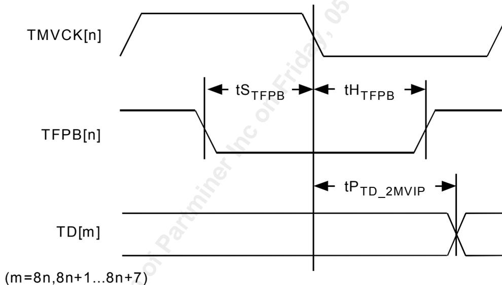
**Figure 48 – Transmit Data & Frame Pulse Timing (8.192 Mbps H-MVIP Mode)**
