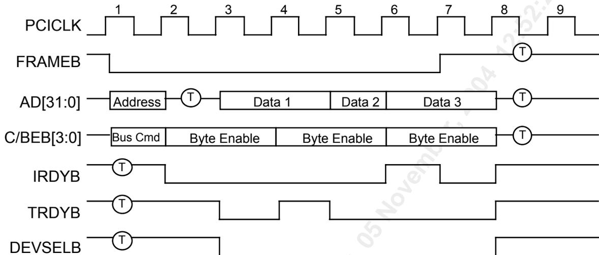
A PCI burst write transaction is shown in Figure 34. The cycle is valid for target and initiator accesses. The target is responsible for incrementing the address for the duration of the data burst. The target is responsible for incrementing the address for the duration of the data burst. The 'T' symbol stands for a turn around cycle. A turn around cycle is required on all signals which can be driven by more than one agent.
