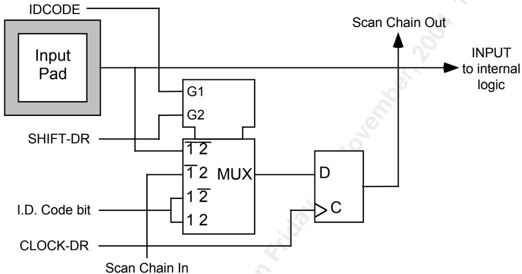
In this diagram and those that follow, **CLOCK-DR** is equal to **TCK** when the current controller state is **SHIFT-DR** or **CAPTURE-DR**, and unchanging otherwise. The multiplexer in the center of the diagram selects one of four inputs, depending on the status of select lines **G1** and **G2**. The ID Code bit is as listed in the table above.
