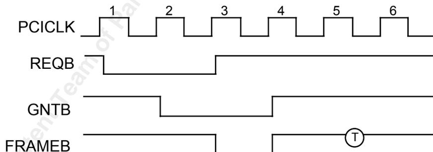
The PCI Initiator Abort Termination Diagram (Figure 38) illustrates the case when the initiator aborts a transaction on the PCI bus.
