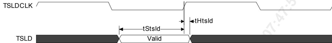
**Table 37 Transmit SONET/SDH Overhead TSLDCLK Interface (Figure 54)**
