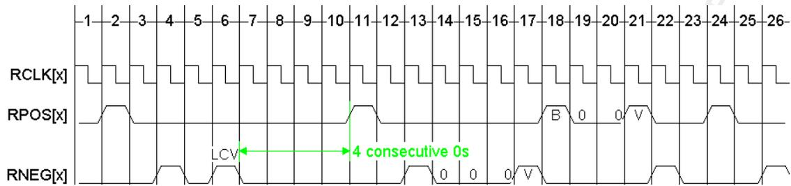
The Receive Bipolar E3 Stream diagram (Figure 20) shows the operation of the ARROW 155 while processing an HDB3-encoded E3 stream on inputs RPOS[x] and RNEG[x]. It is assumed that the first bipolar violation (on RNEG[x]) illustrated corresponds to a valid HDB3 signature (HDB3 Signature Pattern is X00V). A line code violation is declared upon detection of four consecutive zeros in the incoming stream, or upon detection of a bipolar violation, which is not part of a valid HDB3 signature.
