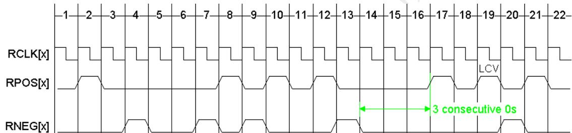
The Receive Bipolar DS3 Stream diagram (Figure 18) shows the operation of the ARROW 155 while processing a B3ZS encoded DS3 stream on inputs RPOS[x] and RNEG[x]. It is assumed that the first bipolar violation (on RNEG[x]) illustrated corresponds to a valid B3ZS signature. A line code violation is declared upon detection of three consecutive zeros in the incoming stream, or upon detection of a bipolar violation which is not part of a valid B3ZS signature.
