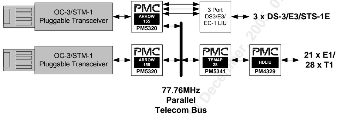
**Figure 4 OC-3/STM-1 Terminal Mux Example #2**
