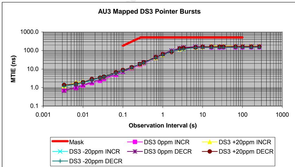
Figure 63 DS3 Pointer Wander MTIE (Phase Transient Pointer Adjustment Burst)
