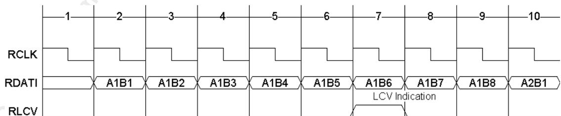
The Receive Unipolar STS-1E Stream diagram (Figure 22) shows the unipolar STS-1E receive signal on the RDATI[x] input. Line code violation indications, detected by an upstream B3ZS decoder, are indicated on input RLCV. RLCV is sampled each bit period. The PMON Line Code Violation Event Counter is incremented each time a logic 1 is sampled on RLCV.
