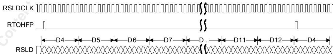
Figure 36 and Figure 37 show the receive section/line DCC (RSLD) functional output timing. When RSLDSEL is set to zero, RSLD and RSLDCLK are carrying the section DCC bytes (D1-D3). When RSLDSEL is set to one, RSLD and RSLDCLK are carrying the line DCC bytes (D4-D12).
