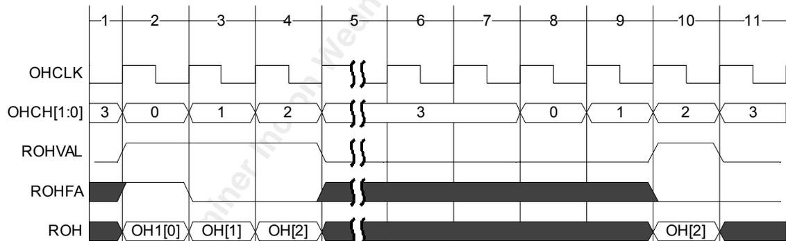
For DS3 overhead extraction, ROHFA is asserted once every 56 bits to mark the X1 bit for each active channel. For each DS3 channel, the order of the overhead bit extraction is shown in Table 12, starting from the top left X1 bit, proceeding to the right, and then from sub-frame 1 to sub-frame 7:
