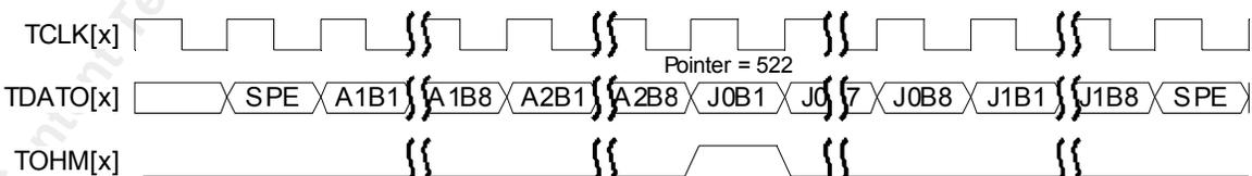
The Transmit Unipolar STS-1E Stream diagram (Figure 28) illustrates the unipolar STS-1E stream generation. The STS-1 SPE along with valid section/line/path overhead bits is contained in TDATO. The TOHM output shown marks the J0 frame boundary (high for all 8 bits of the J0 byte) in the transmit stream.
