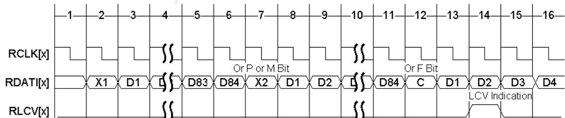
The Receive Unipolar DS3 Stream diagram (Figure 19) shows the complete DS3 receive signal on the RDATI[x] input. Line code violation indications, detected by an upstream B3ZS decoder, are indicated on input RLCV[x]. RLCV[x] is sampled each bit period. The PMON Line Code Violation Event Counter is incremented each time a logic 1 is sampled on RLCV[x].
