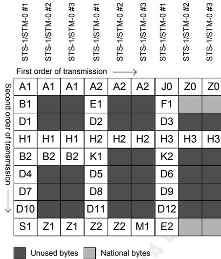
The TRMP serially inputs the line DCC bytes from the TSLD ports. TSLD is selectable to input either the section DCC bytes (D1-D3) or the line DCC bytes (D4-D12). TSLDCLK is the generated output clock used to provide timing for the TSLD port. If TSLD carries the line DCC, TSLDCLK is a nominal 576 kHz clock or if TSLD carries the section DCC, TSLDCLK is a nominal 192 kHz clock. Sampling TTOHFP high identifies the MSB of the first DCC byte on TSLD (D1 or D4).
