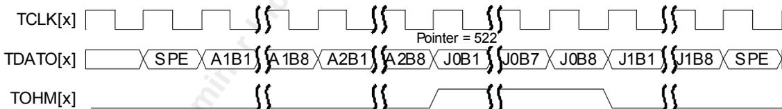
The Transmit Unipolar DS3 Stream diagram (Figure 25) illustrates the unipolar DS3 stream generation. The ATM cell stream, along with valid DS3 overhead bits is contained in TDATO. The TOHM output marks the M-frame boundary (the X1 bit) in the transmit stream. Note that TCLK is a flow through clock from REFCLK[1:0] or an internally generated clock from the DS3 de-synchronizer (D3E3MD) depending on the mode of operation of that channel.
