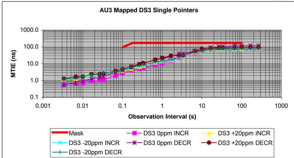
Figure 62 DS3 Pointer Wander MTIE (Burst of 3 Pointer Adjustments)
