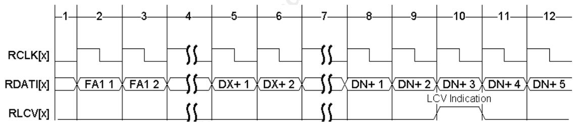
The Receive Unipolar E3 Stream diagram (Figure 21) shows the unipolar E3 receive signal on the RDATI[x] input. Line code violation indications, detected by an upstream HDB3 decoder, are indicated on input RLCV. RLCV is sampled each bit period. The PMON Line Code Violation Event Counter is incremented each time a logic 1 is sampled on RLCV.
