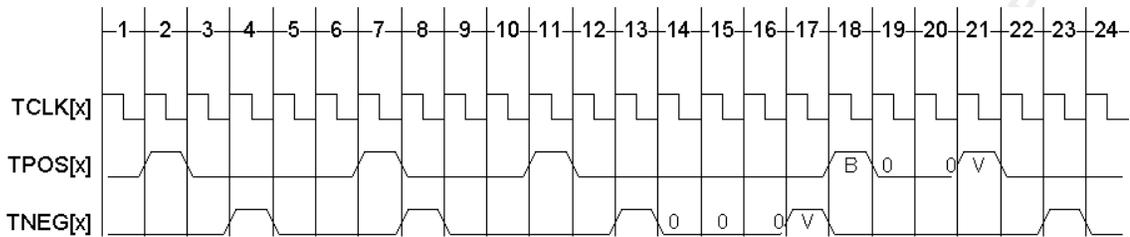
The Transmit Bipolar E3 Stream diagram (Figure 26) illustrates the generation of a bipolar E3 stream. The HDB3 encoded E3 stream is present on TPOS and TNEG (HDB3 Signature Pattern is X00V). These outputs, along with the transmit clock, TCLK, can be directly connected to a E3 line interface unit. Note that TCLK is a flow through clock from REFCLK[1:0] or an internally generated clock from the DS3 de-synchronizer (D3E3MD) depending on the mode of operation of that channel.
