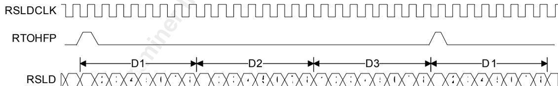
**Figure 37 RTOHFP and RSLD Output Timing (RSLDSEL = 1)**
