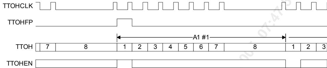
Figure 40 shows the transmit transport overhead (TTOH) functional timings. TTOHCLK is a 5.184 MHz clock generated by gapping a 6.48 MHz clock (33% high duty cycle). 648 bits (9x3x3 bytes) are input on TTOH between two TTOHFP assertions.
