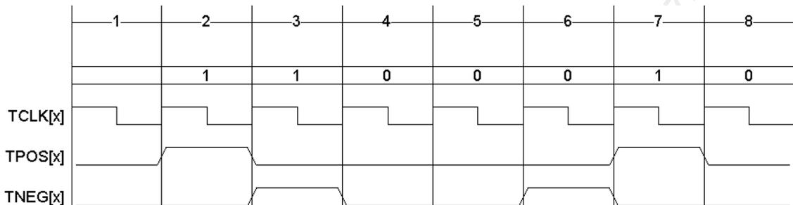
The Transmit Bipolar DS3 Stream diagram (Figure 24) illustrates the generation of a bipolar DS3 stream. The B3ZS encoded DS3 stream is present on TPOS and TNEG. These outputs, along with the transmit clock, TCLK, can be directly connected to a DS3 line interface unit. Note that TCLK is a flow through clock from REFCLK[1:0] or an internally generated clock from the DS3 de-synchronizer (D3E3MD) depending on the mode of operation of that channel.
