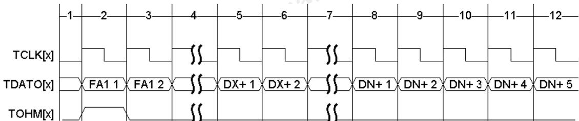
The Transmit Unipolar E3 Stream diagram (Figure 27) illustrates the unipolar E3 stream generation. The ATM cell stream, along with valid E3 overhead bits is contained in TDATO. The TOHM output shown marks the G.832 frame boundary (the first bit of the FA1 frame alignment byte) in the transmit stream. Note that TCLK is a flow through clock from REFCLK[1:0] or an internally generated clock from the DS3 de-synchronizer (D3E3MD) depending on the mode of operation of that channel.
