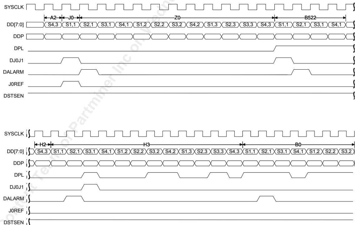
Figure 32 is like Figure 31 except that the J1SQUELCH bit is set to 1 to allow only a single J0 framing pulse on DJ0J1. This mode is useful when the TelecomBus sink is expecting to extract J1 markers from the H1/H2 pointer bytes.
