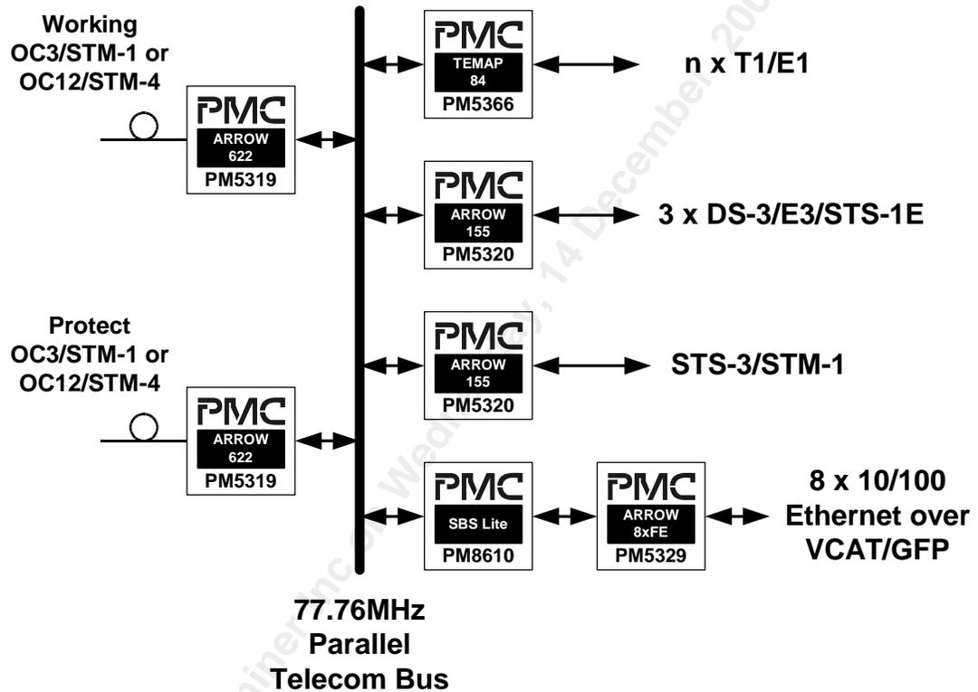
Figure 3 and Figure 4 are both examples of OC-3/STM-1 terminal multiplexers. They illustrate the different PMC-Sierra device combination that allow the insertion/extraction of PDH streams from SONET/SDH.
