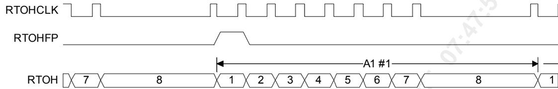
Figure 33 shows the receive transport overhead (RTOH) functional timings in OC-12 mode. RTOHCLK is a 20.736 MHz clock generated by gapping a 25.92 MHz clock (33% high duty cycle). 2592 bits (9x3x12 bytes) are output on RTOH between two RTOHFP assertions.
