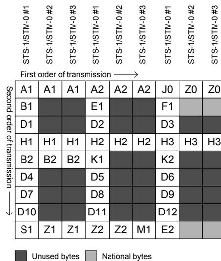
The RRMP optionally serially outputs the line DCC bytes on the RSLD port. RSLD is selectable to output either the section DCC bytes (D1-D3) or the line DCC bytes (D4-D12). RSLDCLK is the generated output clock used to provide timing for the RSLD port. If RSLD carries the line DCC, RSLDCLK is a nominal 576 kHz clock or if RSLD carries the section DCC, RSLDCLK is a nominal 192 kHz clock. Sampling RTOHFP high identifies the MSB of the first DCC byte on RSLD (D1 or D4).
