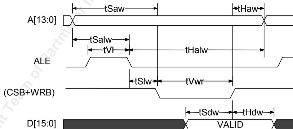
**Table 31 Microprocessor Interface Write Access (Figure 50)**
