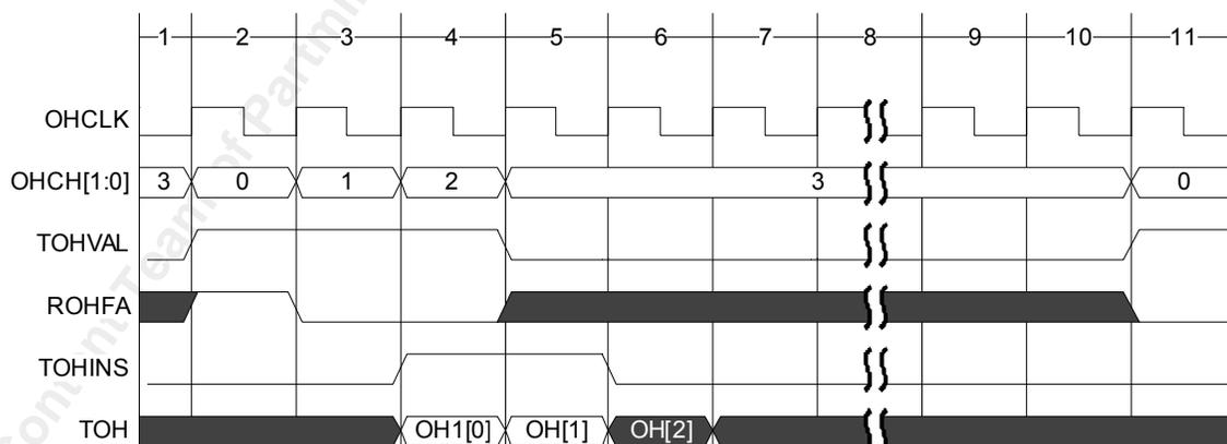
For each DS3 channel, the order of the overhead bit insertion is as shown in Table 16, starting from the top left X1 bit, proceeding to the right, and then from sub-frame 1 to sub-frame 7. TOHFA is asserted once every 56 bits to mark the X1 bit for each active channel.
