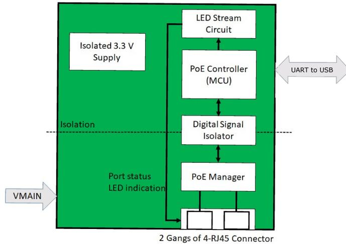
Input supply to the board is DC and it can be fed through the  $V_{IN}$  connector (see [electrical characteristics \(see page 7\)](#) for the input voltage range). The auxiliary power supply (5 V and 3.3 V) for the PD69208M /PD69208T4/PD69204T4 is generated internally and the auxiliary power supply (3.3 V) for the PD69200 MCU is generated using a 3.3 V isolated DC – DC converter.
