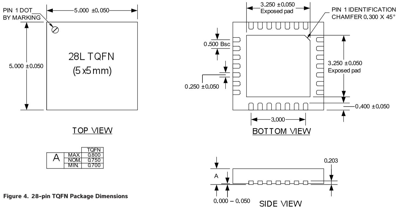
Figure 4. 28-pin TQFN Package Dimensions
