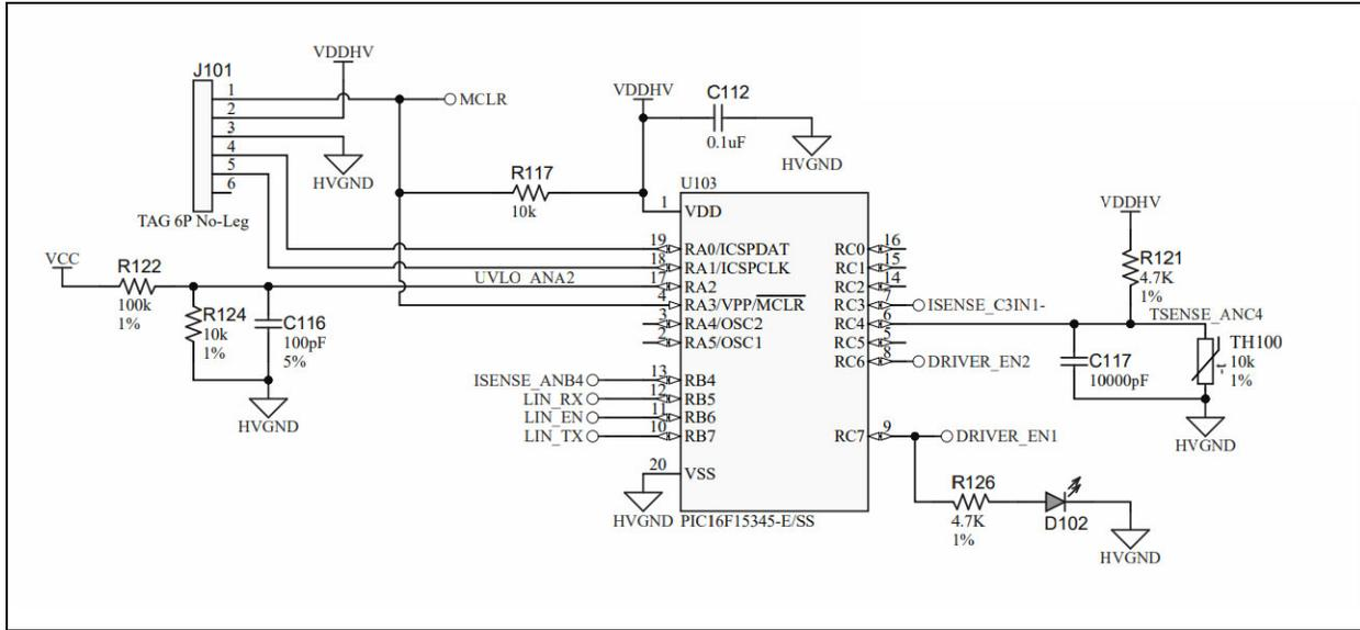
**FIGURE 2-6:** High-Voltage Auxiliary E-Fuse Controller Schematic.
