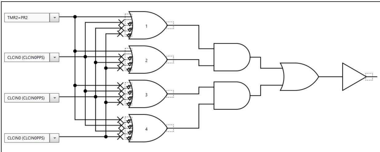
**FIGURE 2-10:** Configurable Logic Cell 4.
