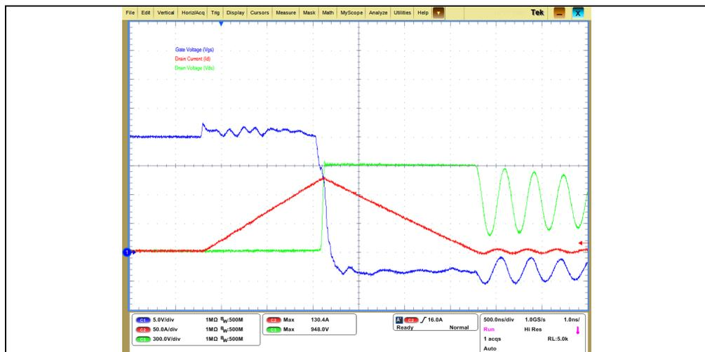
**FIGURE 2-44:** High-Voltage Auxiliary E-Fuse Variant B Short-Circuit Measurement.
