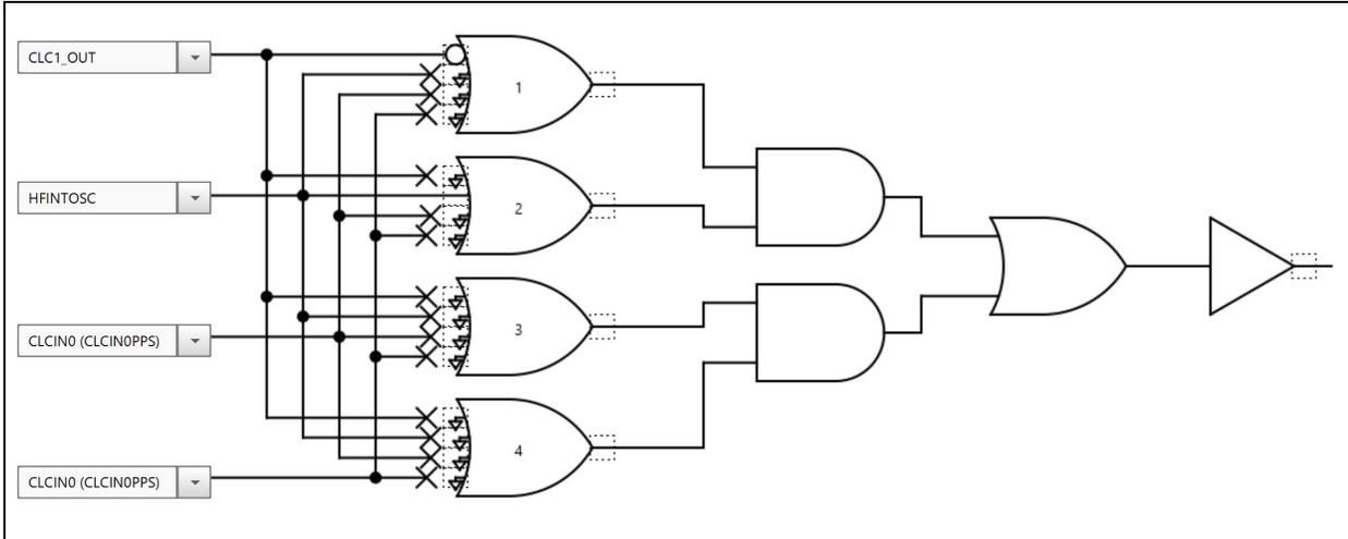
**FIGURE 2-9:** Configurable Logic Cell 3.
