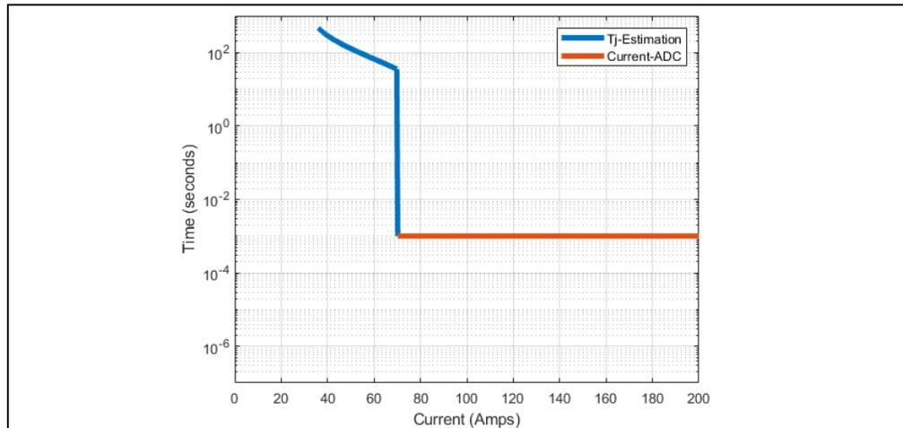
**FIGURE 2-30:** TCC Curve with Over-Current Detection.
