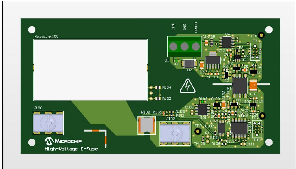
**FIGURE 1-6:** High-Voltage Auxiliary E-Fuse PCB Assembly (Top View).
