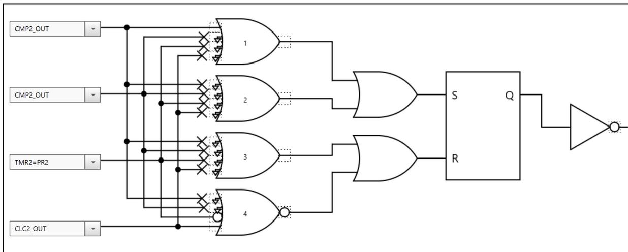
**FIGURE 2-7:** Configurable Logic Cell 1.
