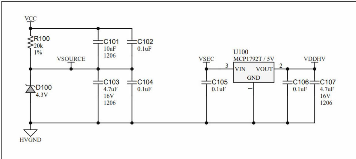
**FIGURE 2-4:** Secondary Power Schematic.
