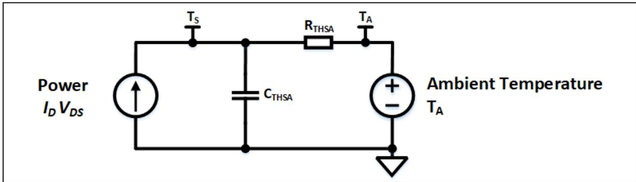
**FIGURE 2-24:** HS Thermal Model.
