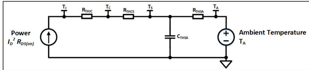
**FIGURE 2-28:** TCC Thermal Model.
