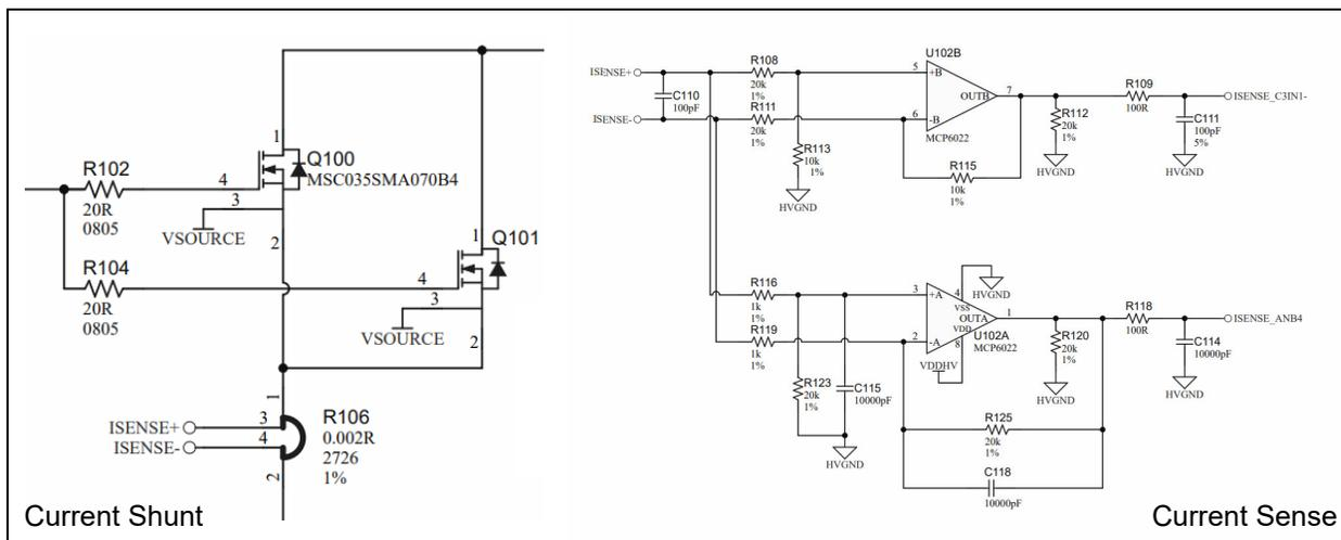
**FIGURE 2-11:** Current Shunt (Left) and Current Sense (Right) Schematics.
