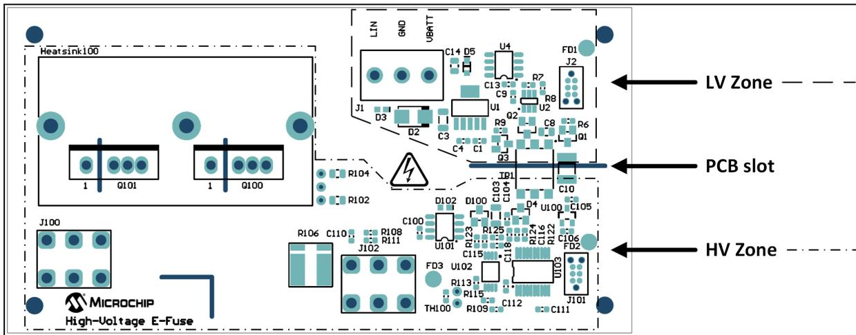
FIGURE 2-18: PCB Creepage.
