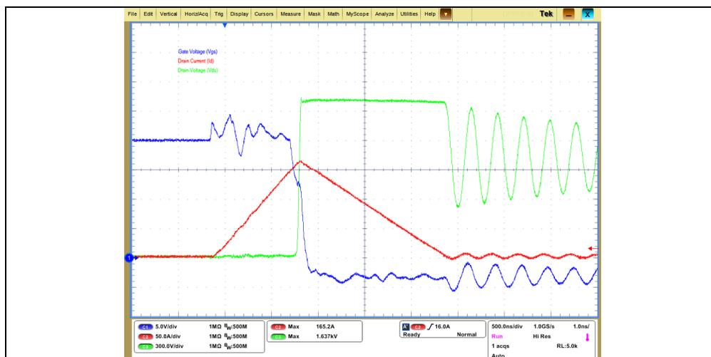
**FIGURE 2-47:** High-Voltage Auxiliary E-Fuse Variant E Short-Circuit Measurement.
