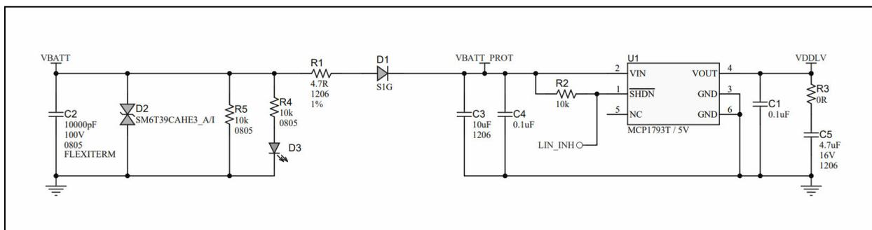
**FIGURE 2-2:** Battery Input Circuit.
