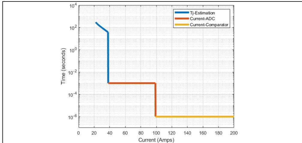
**FIGURE 2-35:** TCC Curve, Variant E (800V, 20A).
