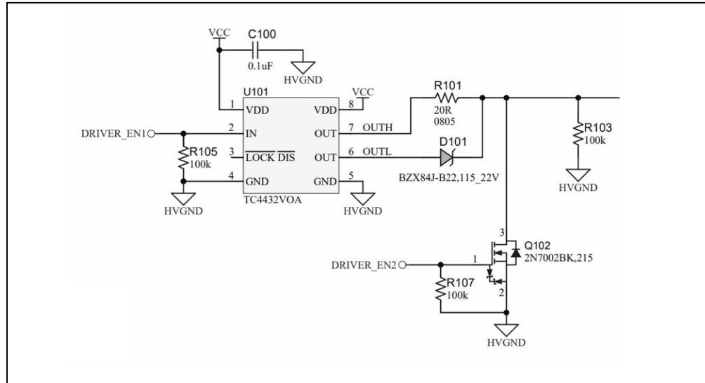
**FIGURE 2-12:** Gate Drive Schematic.
