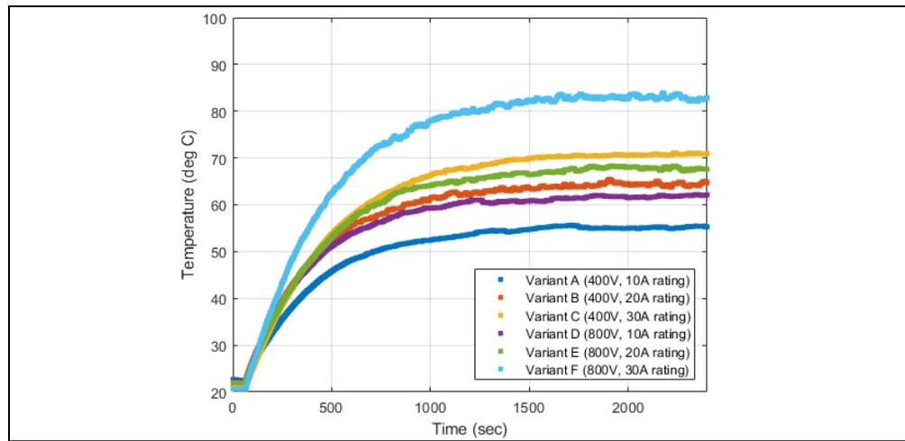
**FIGURE 2-23:** Heat Sink Temperature at Rated Current.
