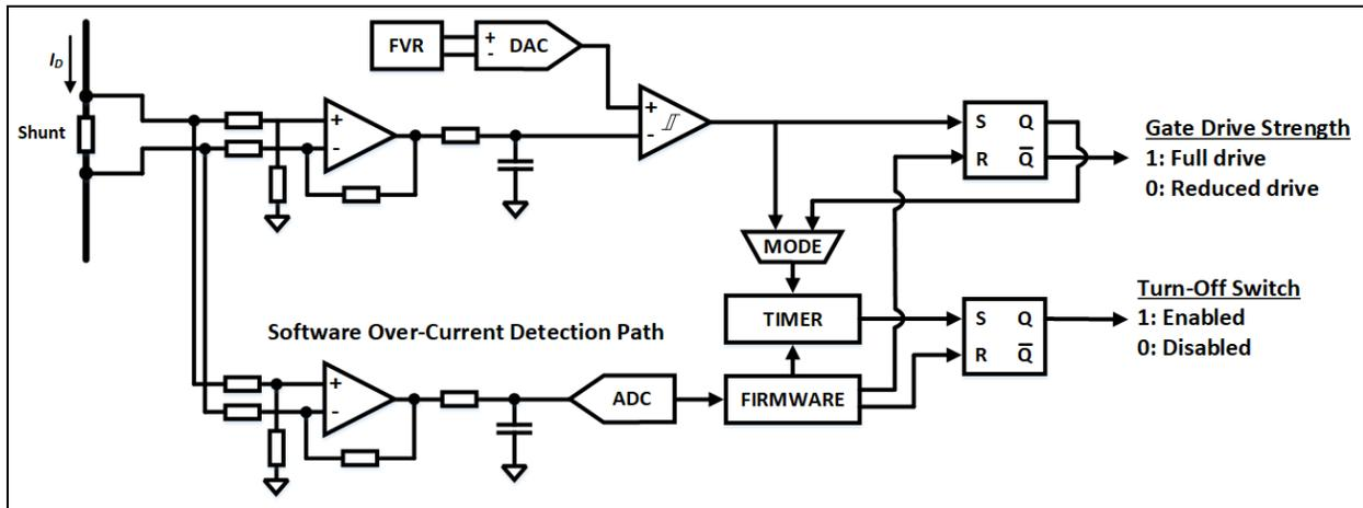
**FIGURE 1-4:** Hardware Short-Circuit Detection Path.
