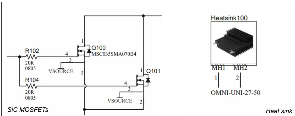
**FIGURE 2-13:** SiC MOSFETs (Left) and Heat Sink (Right) Schematic.
