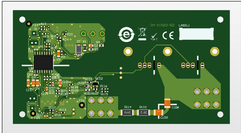
**FIGURE 1-7:** High-Voltage Auxiliary E-Fuse PCB Assembly (Bottom View).
