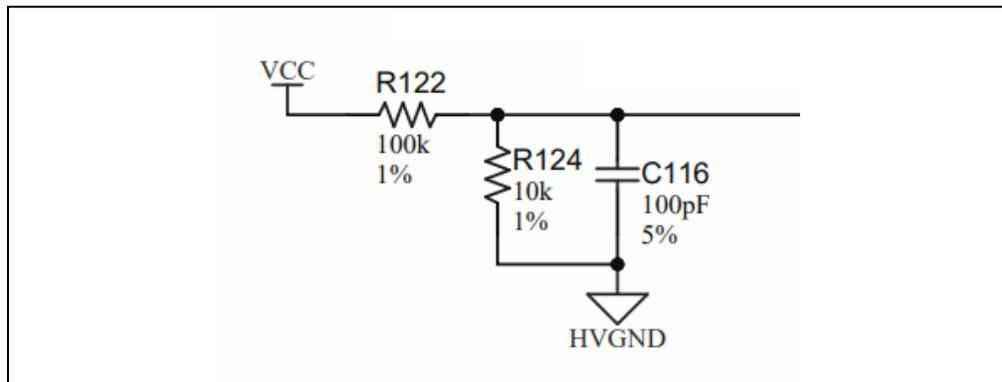
**FIGURE 2-16:** VCC Monitor Schematic.
