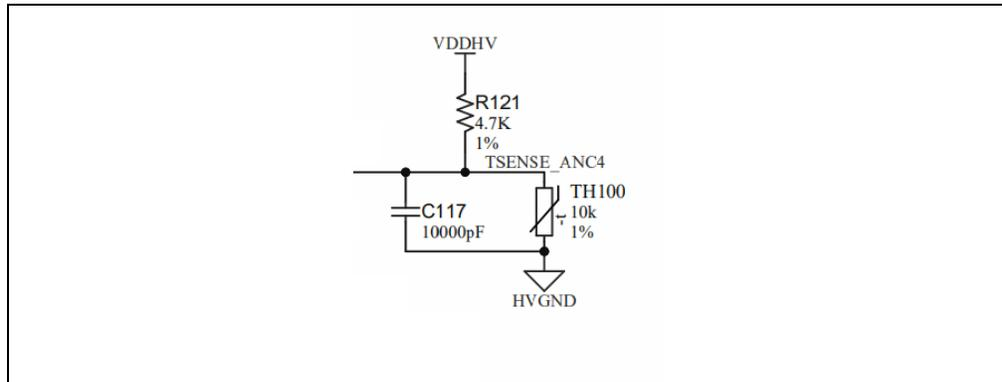
**FIGURE 2-15:** Temperature Sense Schematic.
