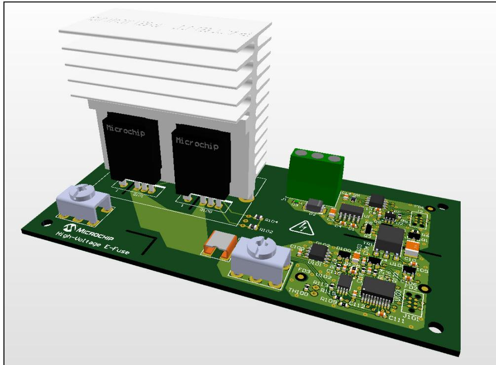
**FIGURE 1-5:** High-Voltage Auxiliary E-Fuse PCB Assembly (Top 3D View).
