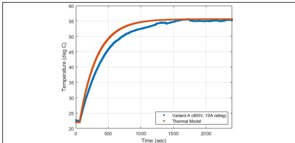
**FIGURE 2-26:** 25 mm Heat Sink RC Thermal Model Transient Response.
