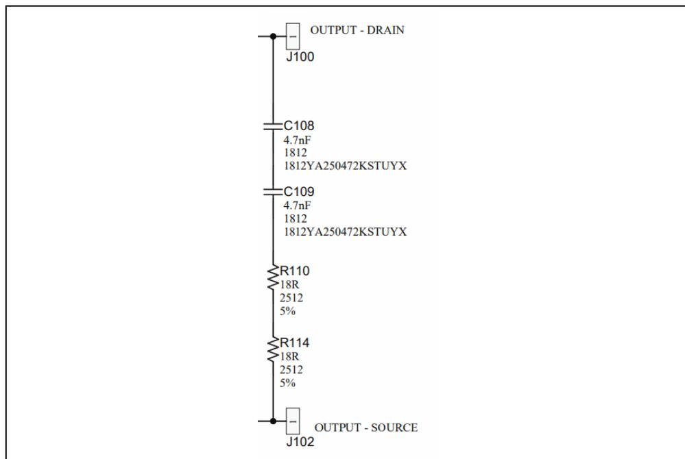
**FIGURE 2-14:** Snubber Schematic.
