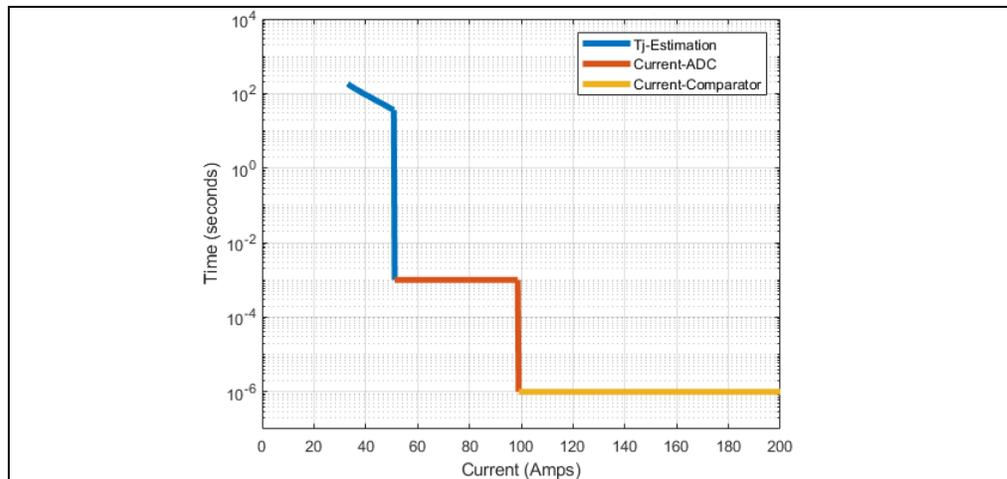
**FIGURE 2-36:** TCC Curve, Variant F (800V, 30A).
