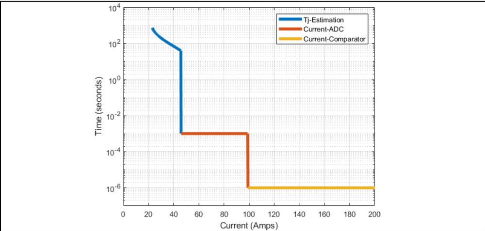
FIGURE 2-33: TCC Curve, Variant C (400V, 30A).
