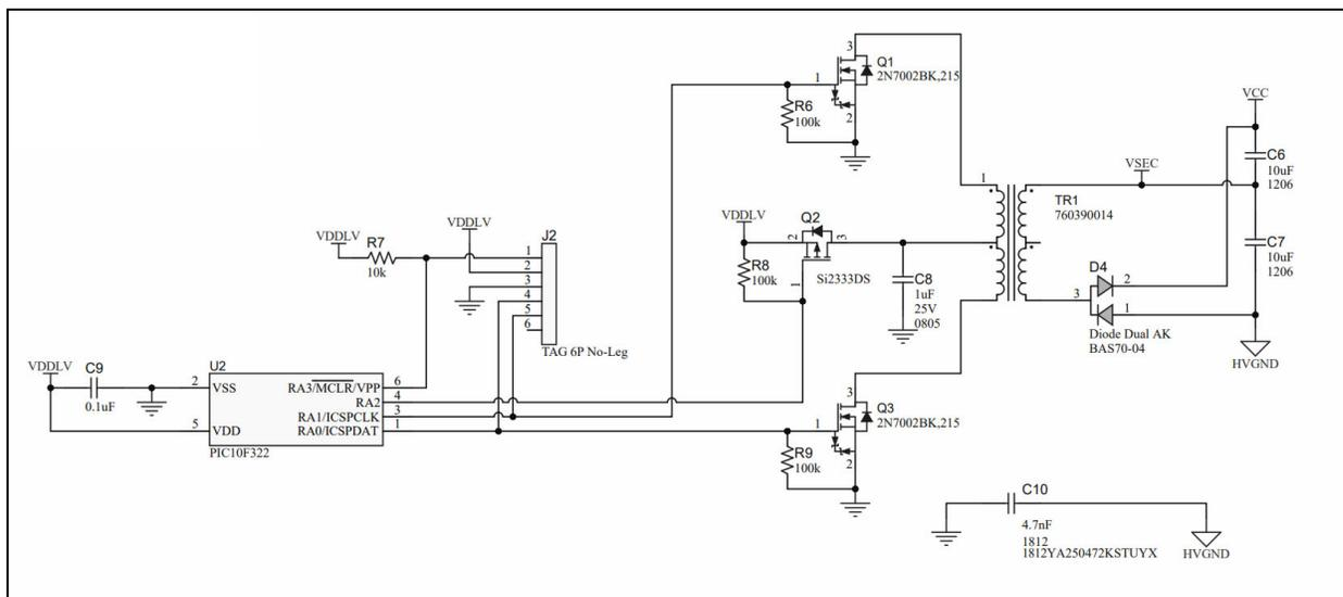
**FIGURE 2-3:** Push-Pull Converter Schematic.
