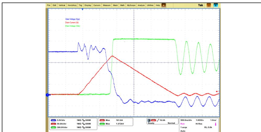
**FIGURE 2-48:** High-Voltage Auxiliary E-Fuse Variant F Short-Circuit Measurement.
