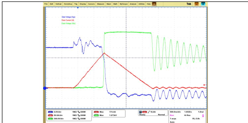
**FIGURE 2-46:** High-Voltage Auxiliary E-Fuse Variant D Short-Circuit Measurement.
