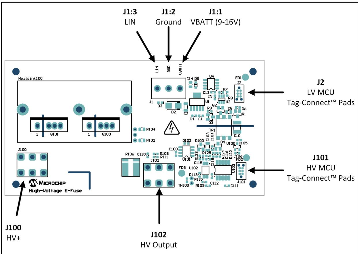
**FIGURE 1-2:** Pinout.
