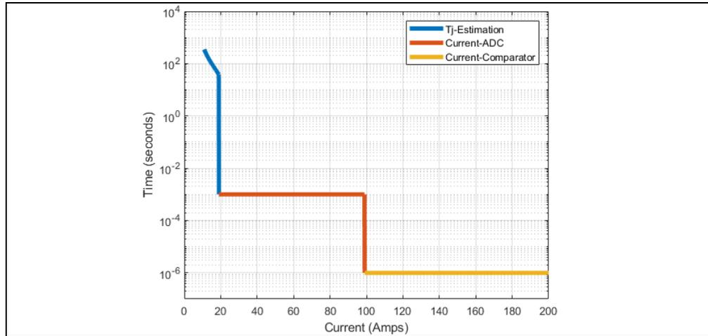
**FIGURE 2-34:** TCC Curve, Variant D (800V, 10A).
