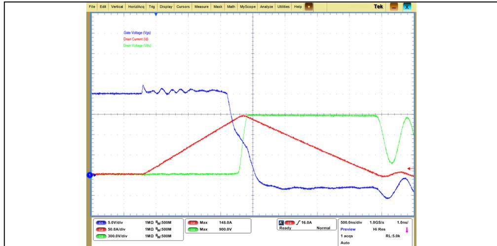
**FIGURE 2-45:** High-Voltage Auxiliary E-Fuse Variant C Short-Circuit Measurement.
