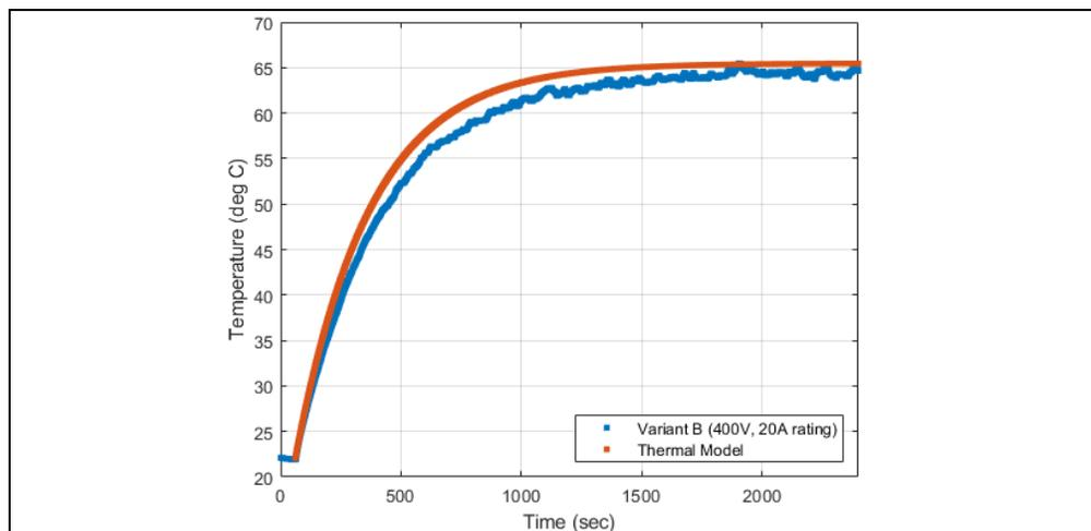
**FIGURE 2-27:** 50 mm Heat Sink RC Thermal Model Transient Response.
