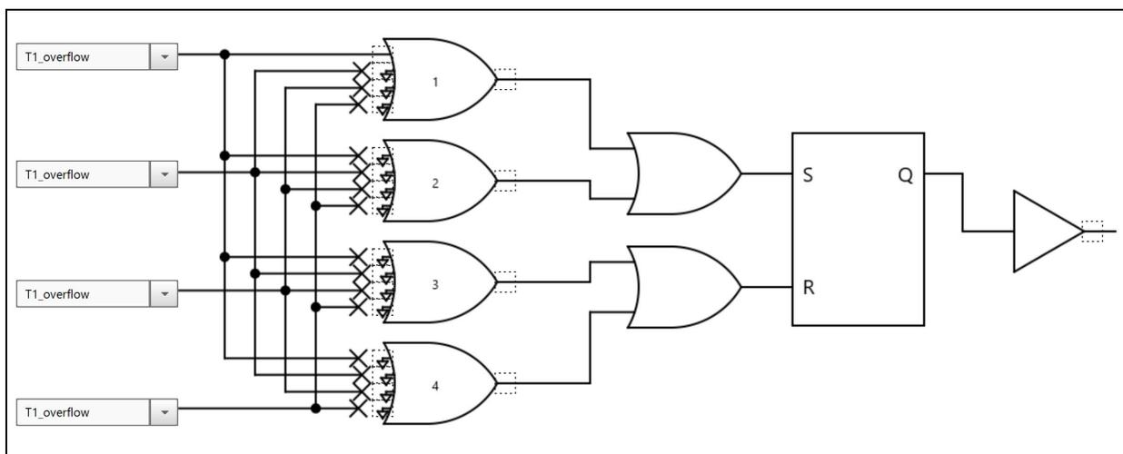
**FIGURE 2-8:** Configurable Logic Cell 2.
