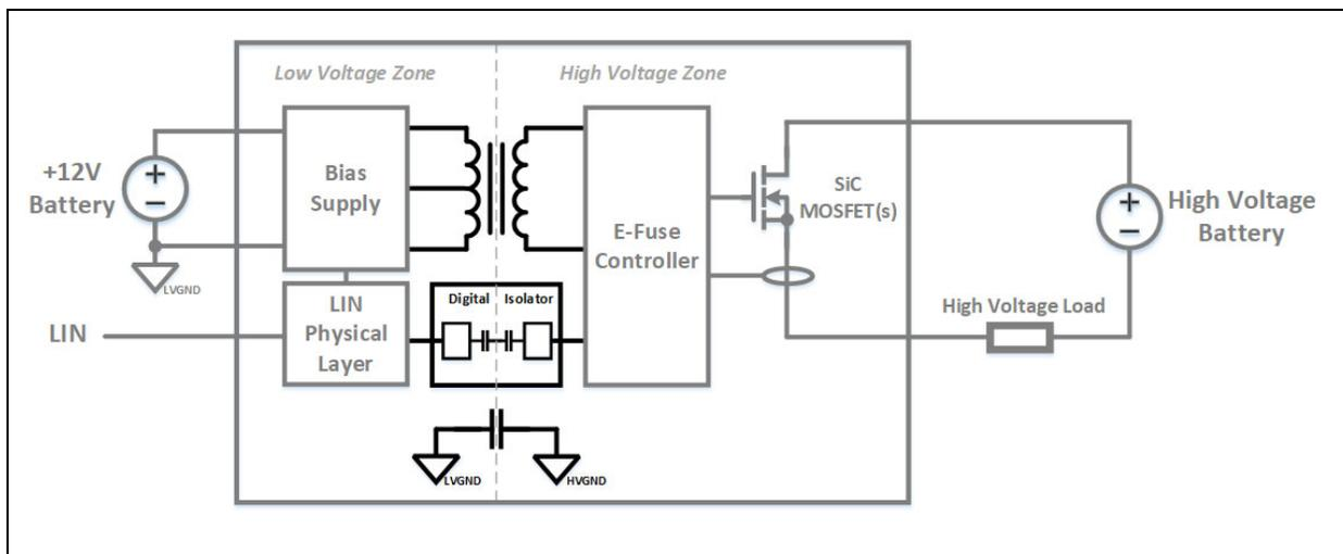
**FIGURE 2-17:** Isolation of Components.
