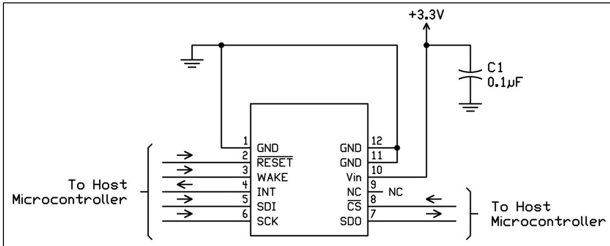
FIGURE 2-5: MRF24J40MD/ME SCHEMATIC
