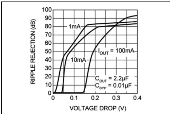
**FIGURE 2-8:** Power Supply Ripple Rejection vs. Voltage Drop.
