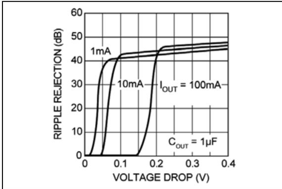
**FIGURE 2-7:** Power Supply Ripple Rejection vs. Voltage Drop.
