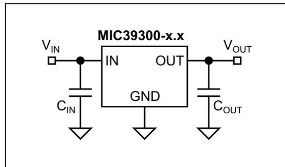
**FIGURE 4-1:** Capacitor Requirements.
