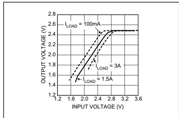
**FIGURE 2-5:** Dropout Characteristics.
