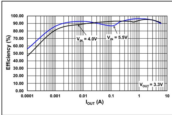
**FIGURE 2-8:** Efficiency vs. Load Current ( $V_{OUT} = 3.3V$ ).
