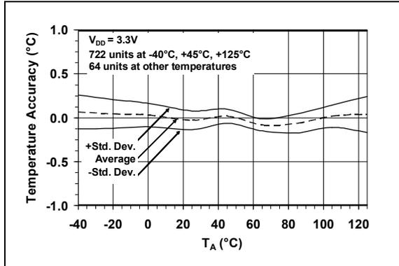
**FIGURE 2-1:** Temperature Accuracy.
