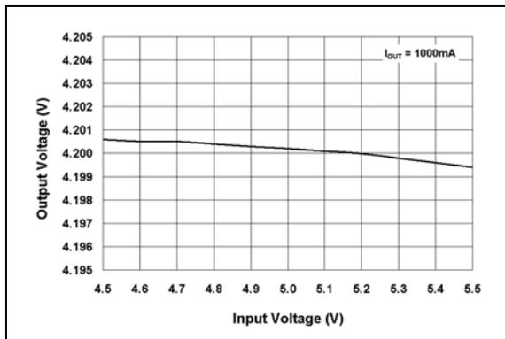
**FIGURE 2-2:** Output Voltage vs. Input Voltage (MCP73826-4.2).
