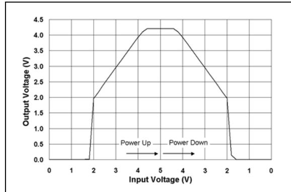
**FIGURE 2-12:** Power-Up / Power-Down.
