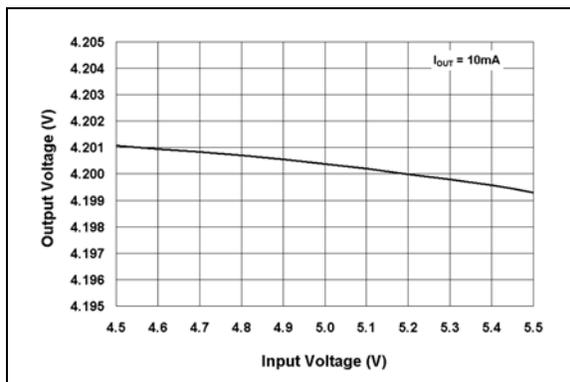
**FIGURE 2-3:** Output Voltage vs. Input Voltage (MCP73826-4.2).
