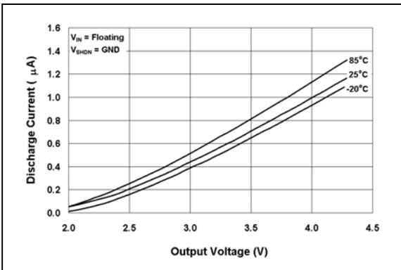
**FIGURE 2-8:** Output Reverse Leakage Current vs. Output Voltage.
