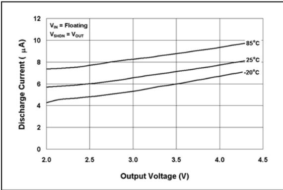
**FIGURE 2-7:** Output Reverse Leakage Current vs. Output Voltage.
