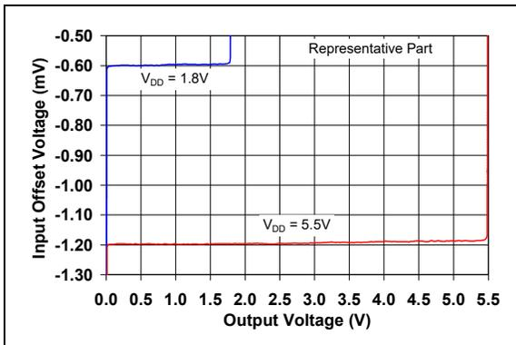
**FIGURE 2-3:** Input Offset Voltage vs. Output Voltage.
