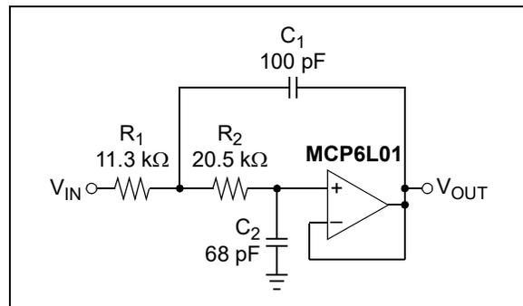
FIGURE 4-5: Bessel Filter.
