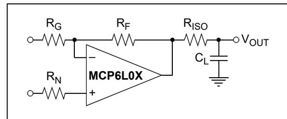
FIGURE 4-2: Output Resistor,  $R_{ISO}$ , Stabilizes Large Capacitive Loads.
