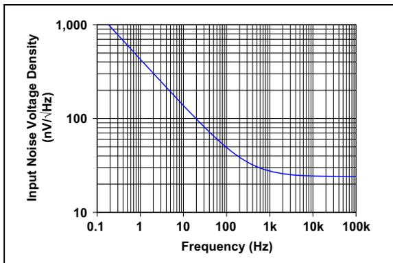
**FIGURE 2-9:** Input Noise Voltage Density vs. Frequency.
