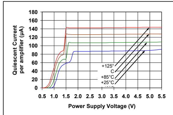
**FIGURE 2-11:** Quiescent Current vs. Power Supply Voltage.
