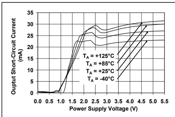
**FIGURE 2-21:** Output Short Circuit Current vs. Supply Voltage.
