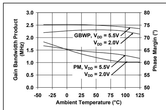
**FIGURE 2-18:** Gain Bandwidth Product, Phase Margin vs. Temperature.
