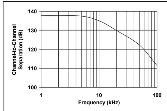
**FIGURE 2-24:** Channel-to-Channel Separation vs. Frequency (MCP6272 and MCP6274).
