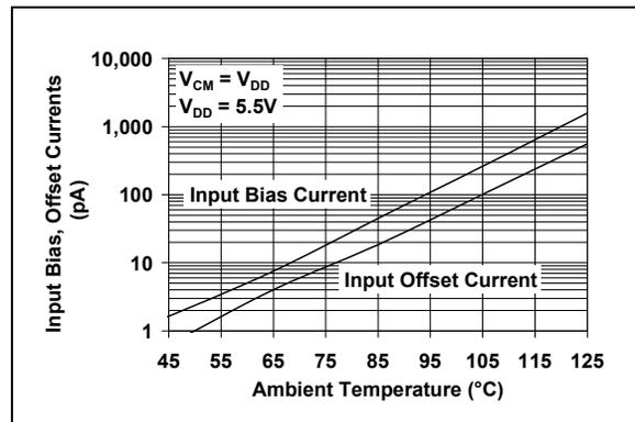
**FIGURE 2-11:** Input Bias, Input Offset Currents vs. Temperature.
