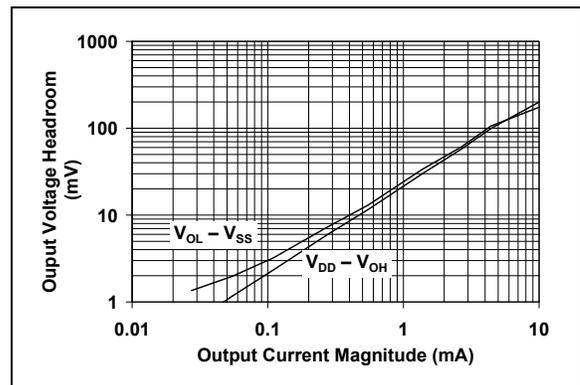
**FIGURE 2-17:** Output Voltage Headroom vs. Output Current Magnitude.
