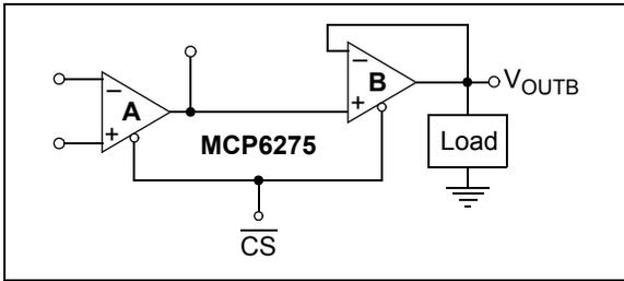
**FIGURE 4-10:** Isolating the Load with a Buffer.
