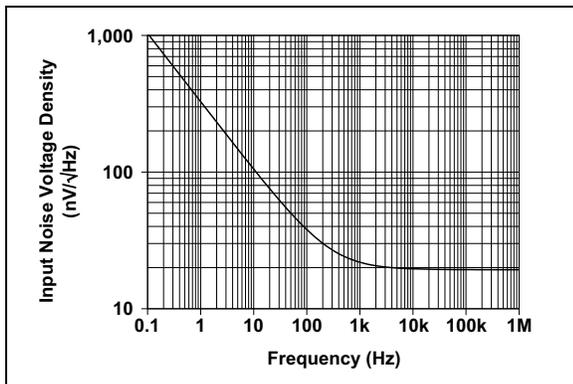
**FIGURE 2-20:** Input Noise Voltage Density vs. Frequency.
