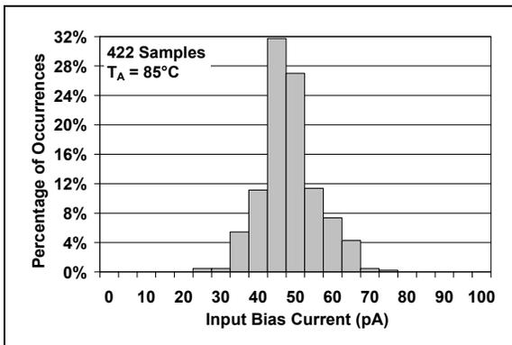
**FIGURE 2-2:** Input Bias Current at  $T_A = +85^\circ\text{C}$ .
