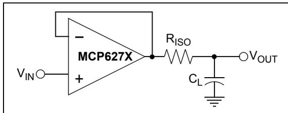
**FIGURE 4-3:** Output Resistor,  $R_{ISO}$  stabilizes large capacitive loads.
