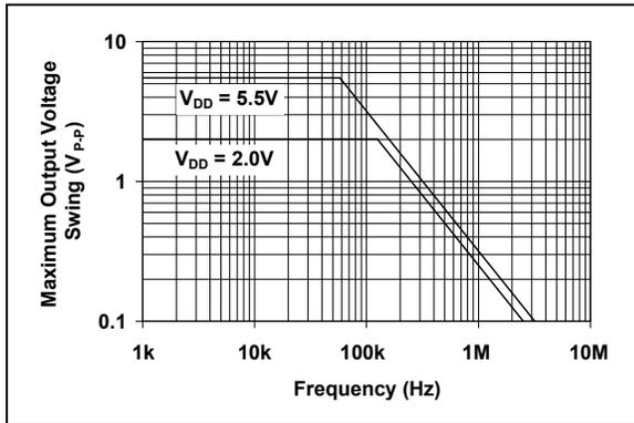
**FIGURE 2-19:** Maximum Output Voltage Swing vs. Frequency.
