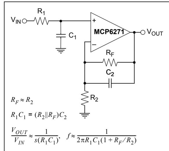
**FIGURE 4-9:** Non-Inverting Integrator.
