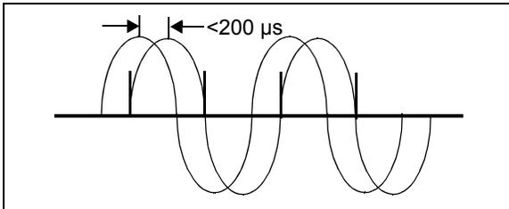
**FIGURE 5-7:** Zero Crossing Detection Operation (Non-Inverted, Pulsed).
