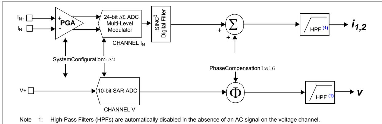
**FIGURE 5-1:** Channels 1 or 2 ( $I_N$  and  $V$ ) Input-Signal Flow.
