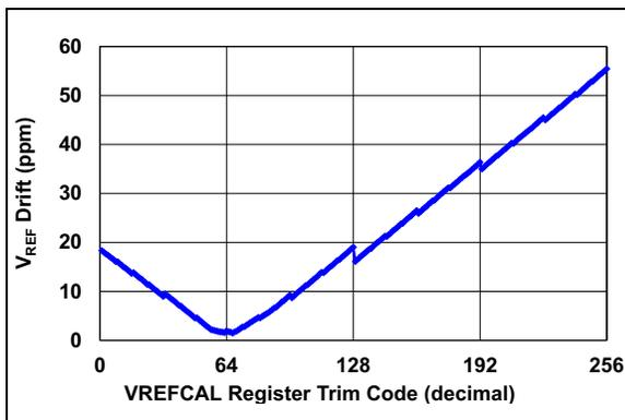
**FIGURE 6-1:**  $V_{REF}$  Tempco vs. VREFCAL Trimcode Chart.
