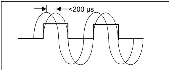
**FIGURE 5-6:** Zero Crossing Detection Operation (Non-Inverted, Non-Pulse).
