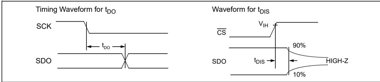
**FIGURE 1-4:** Timing Waveforms.
