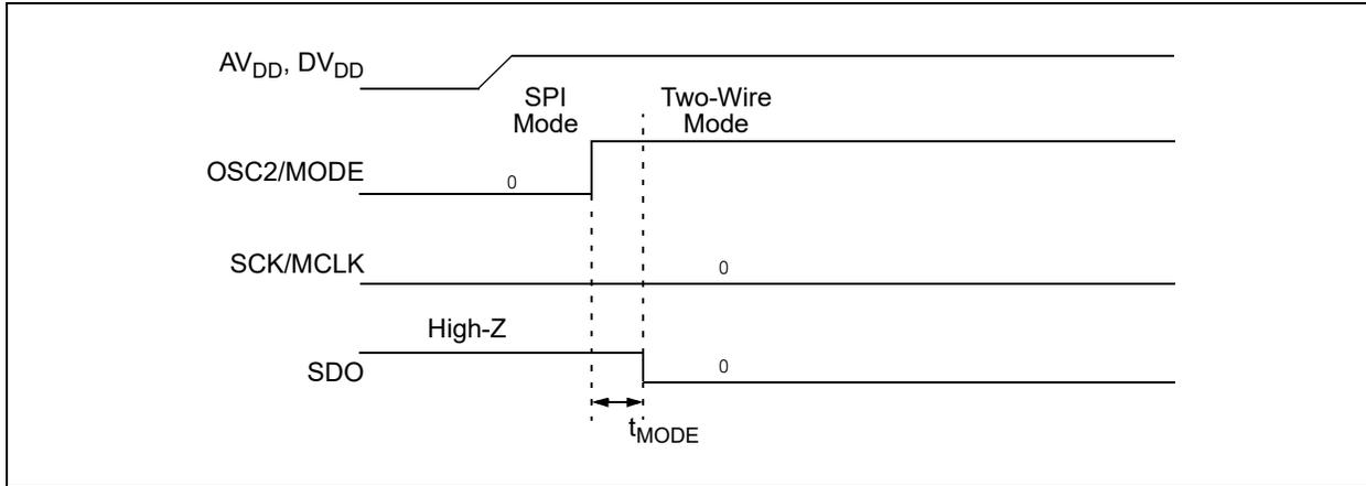
**FIGURE 1-5:** Entering Two-Wire Interface Mode Timing Diagram.
