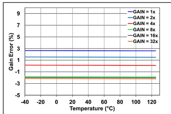
**FIGURE 2-35:** Gain Error vs. Temperature vs. Gain.
