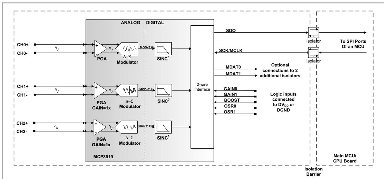
**FIGURE 7-1:** MCP3919 Two-Wire Interface Typical Application Schematic.
