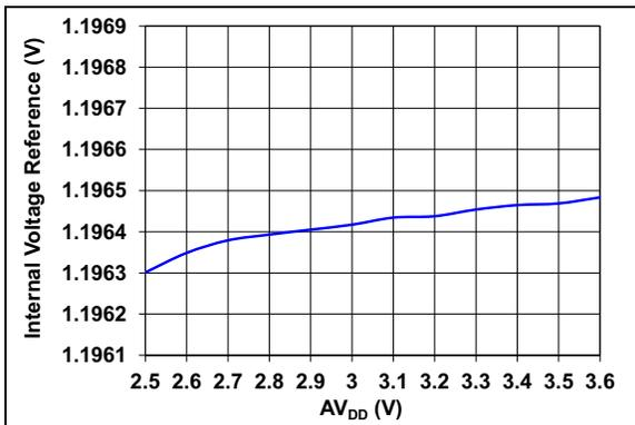
**FIGURE 2-37:** Internal Voltage Reference vs. Supply Voltage.
