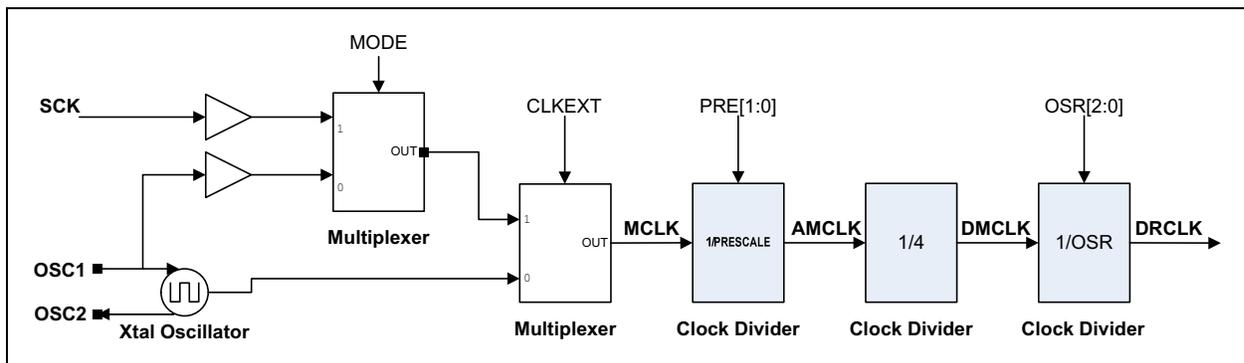
**FIGURE 4-1:** Clock Sub-Circuitry.
