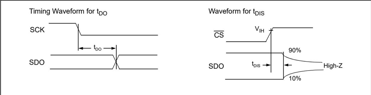
FIGURE 1-4: Timing Waveforms.
