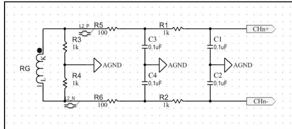
**FIGURE 7-7: Second-Order Anti-Aliasing Filter for Rogowski Coil-Based Designs.**
