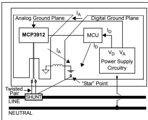
**FIGURE 7-5:** Connection Diagram.
