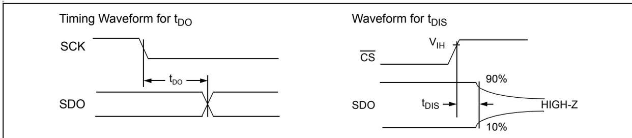
**FIGURE 1-4:** Timing Waveforms.
