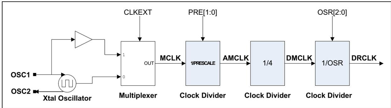
**FIGURE 4-1:** Clock Sub-Circuitry.
