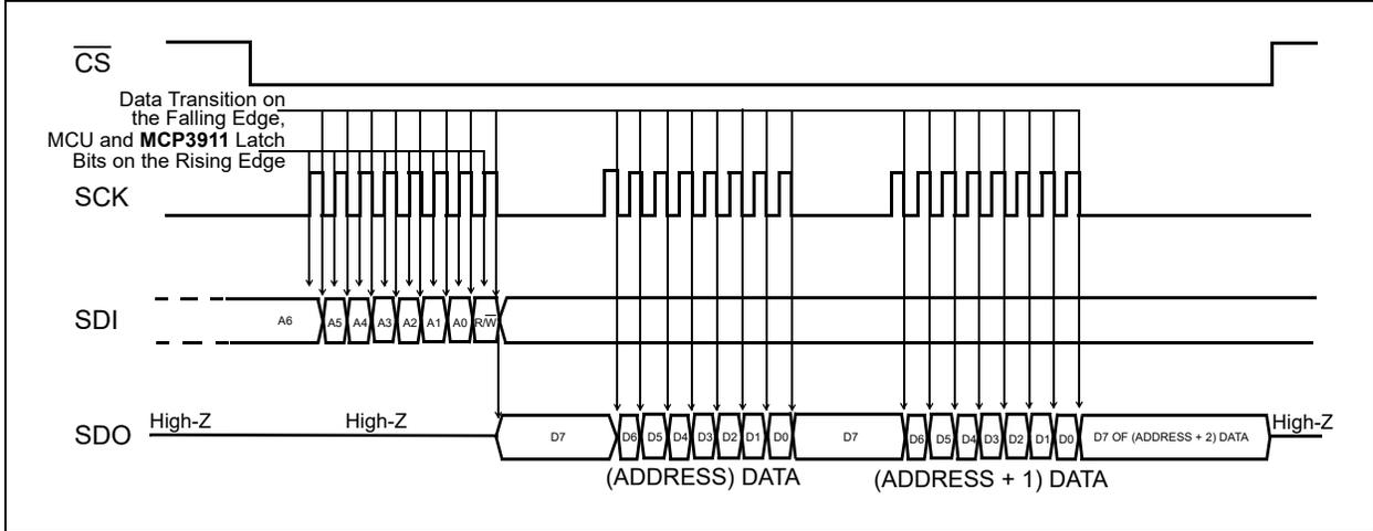
**FIGURE 6-4:** Device Read (SPI Mode 0,0 – SCK Idles Low).
