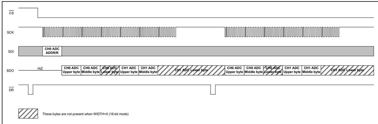
**FIGURE 6-7:** Typical Continuous Read Communication (SPI Mode 1,1).
