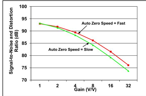
**FIGURE 2-22:** SINAD vs. GAIN vs. AZ Speed Chart.
