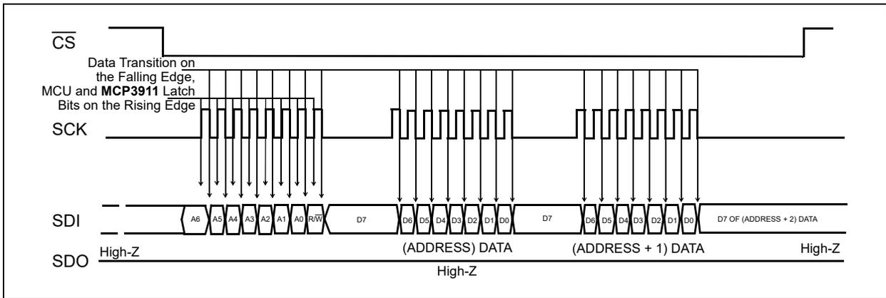
**FIGURE 6-5:** Device Write (SPI Mode 0,0 – SCK Idles Low).
