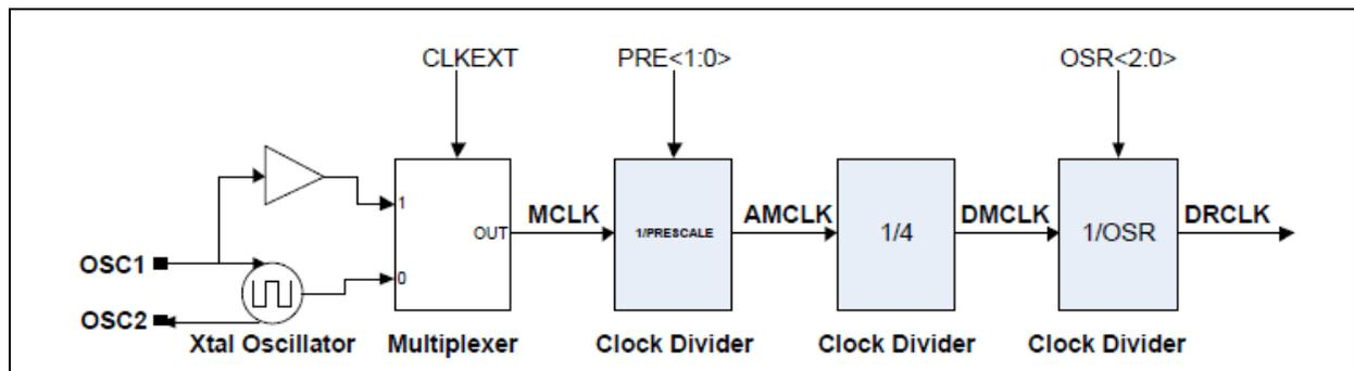
**FIGURE 4-1:** Clock Sub-Circuitry.
