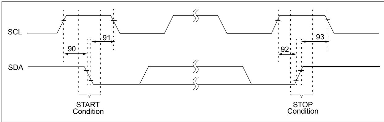
FIGURE 2-4: I<sup>2</sup>C™ BUS DATA TIMING
