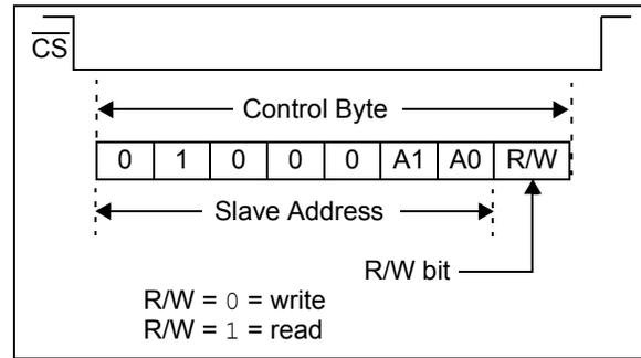
**FIGURE 1-4: I<sup>2</sup>C™ ADDRESSING REGISTERS**
