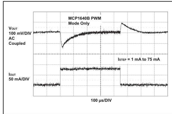
**FIGURE 2-22:** MCP1640B 3.3V  $V_{OUT}$  Load Transient Waveforms.
