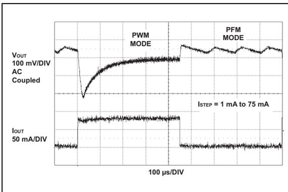
**FIGURE 2-21:** MCP1640 3.3V  $V_{OUT}$  Load Transient Waveforms.
