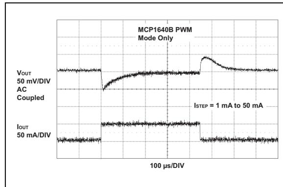
**FIGURE 2-23:** MCP1640B 2.0V  $V_{OUT}$  Load Transient Waveforms.
