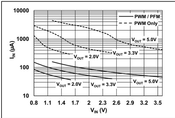
**FIGURE 2-13:** Input No Load Current vs.  $V_{IN}$ .
