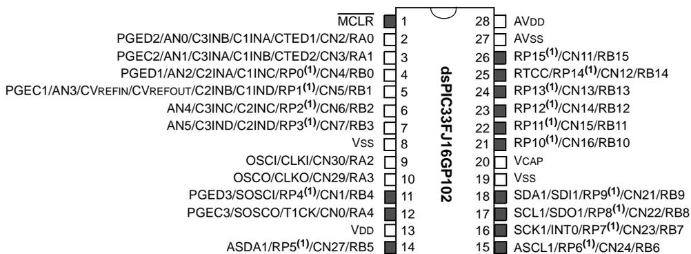
**Note 1:** The RPN pins can be used by any remappable peripheral. See [Table 1](#) for the list of available peripherals.
