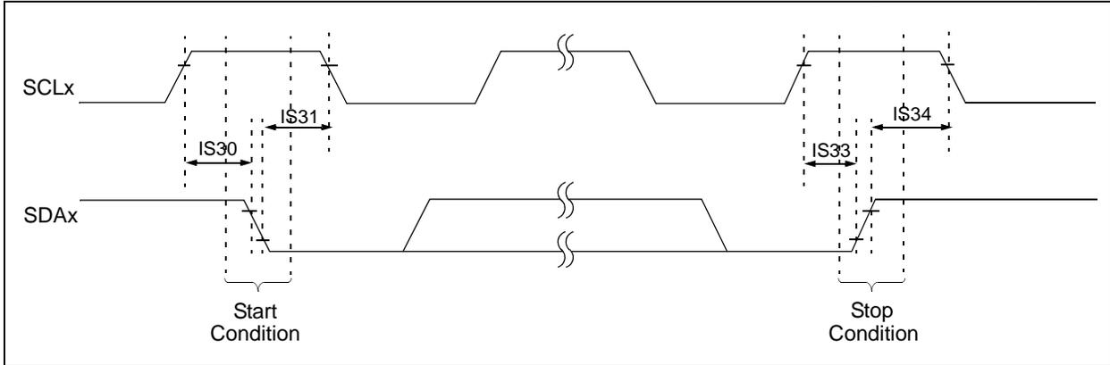
FIGURE 26-22: I2Cx BUS DATA TIMING CHARACTERISTICS (SLAVE MODE)
