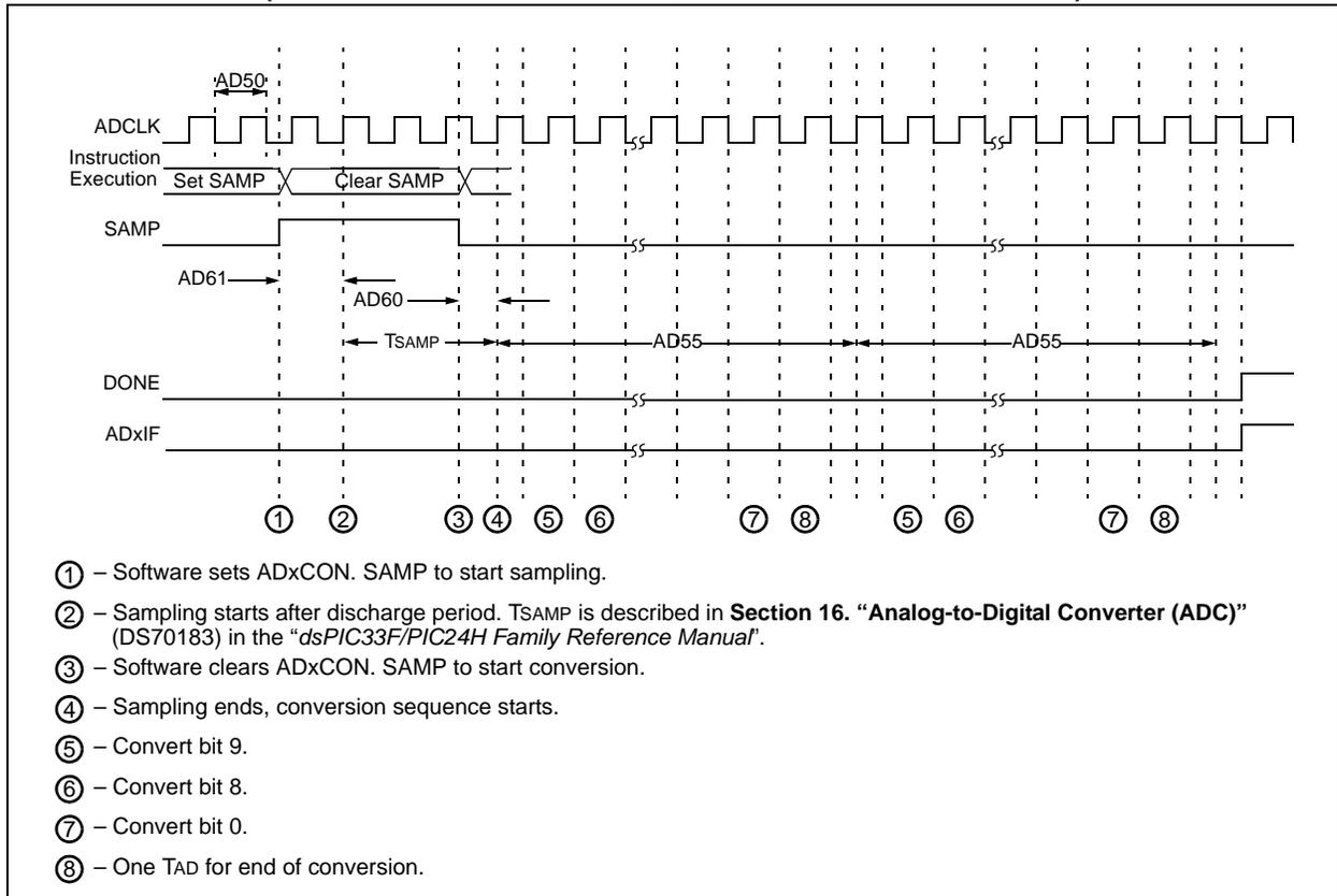
**FIGURE 26-24: ADC CONVERSION TIMING CHARACTERISTICS (CHPS<1:0> = 01, SIMSAM = 0, ASAM = 1, SSRC<2:0> = 111, SAMC<4:0> = 00001)**
