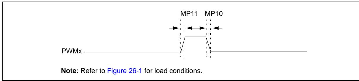
**TABLE 26-28: MOTOR CONTROL PWM MODULE TIMING REQUIREMENTS**
