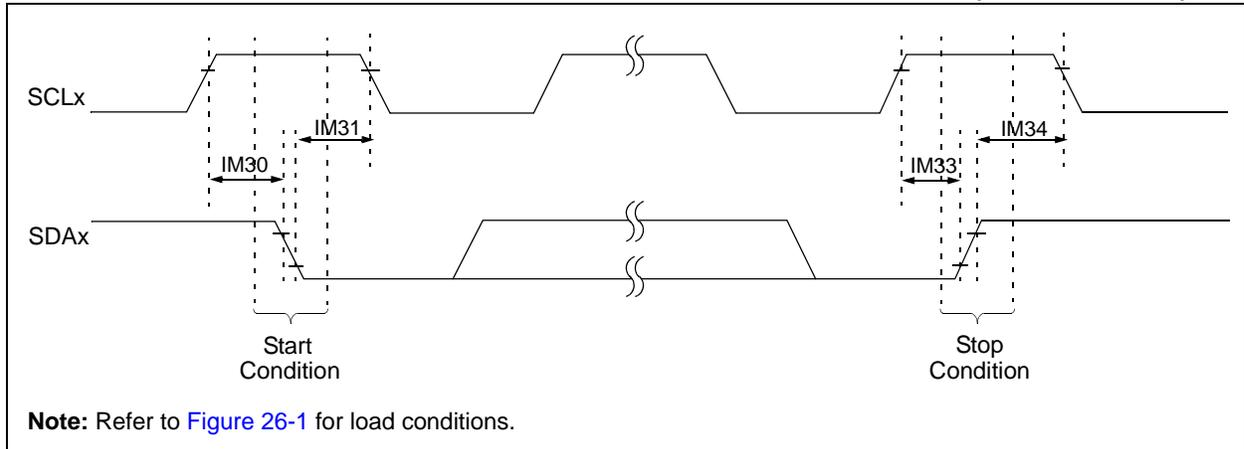
**FIGURE 26-20: I2Cx BUS DATA TIMING CHARACTERISTICS (MASTER MODE)**
