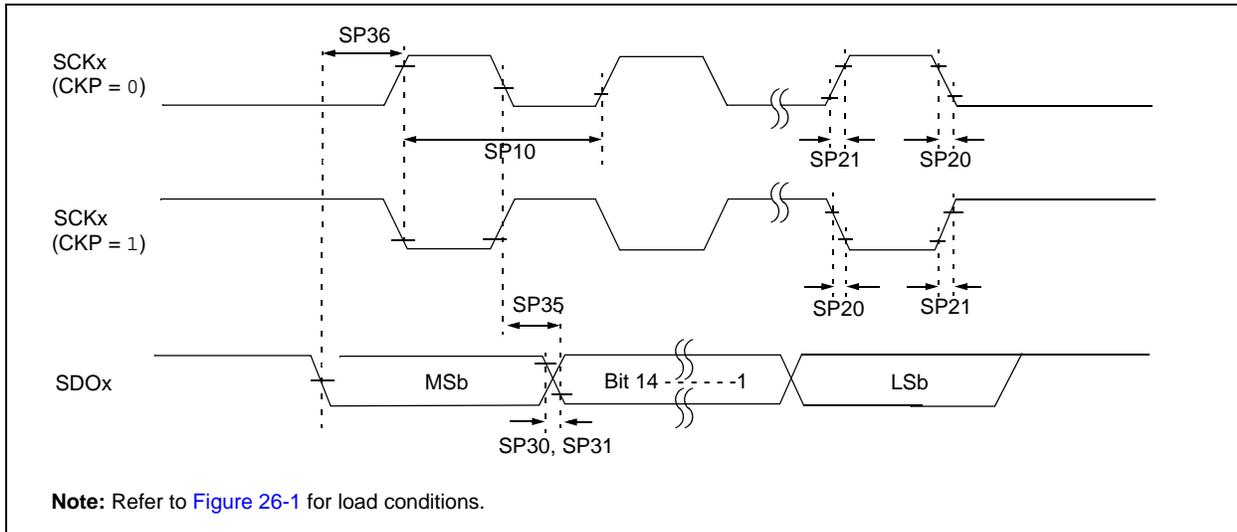
**TABLE 26-30: SPIx MASTER MODE (HALF-DUPLEX, TRANSMIT ONLY) TIMING REQUIREMENTS**
