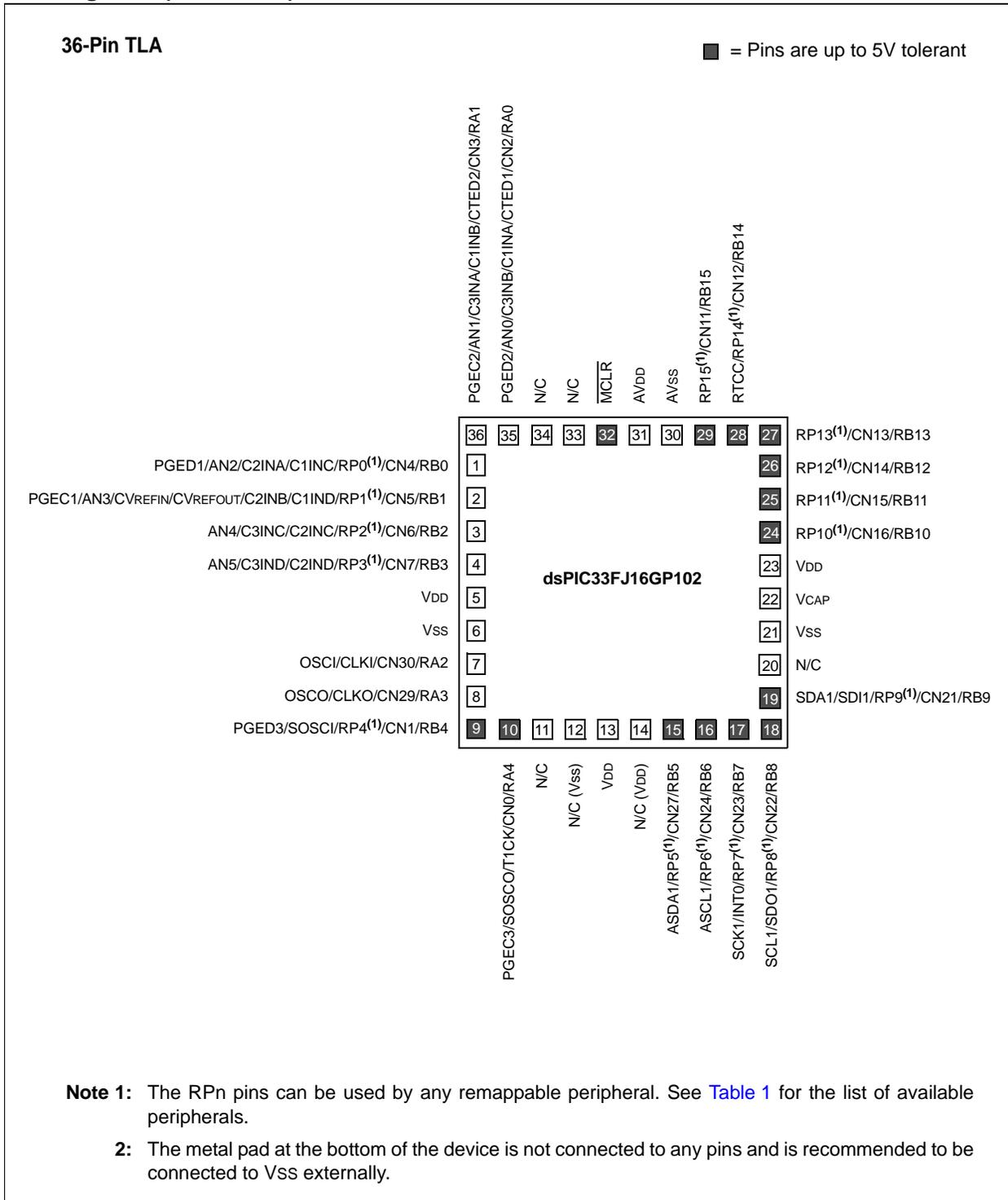
**Note 1:** The RPN pins can be used by any remappable peripheral. See [Table 1](#) for the list of available peripherals.
