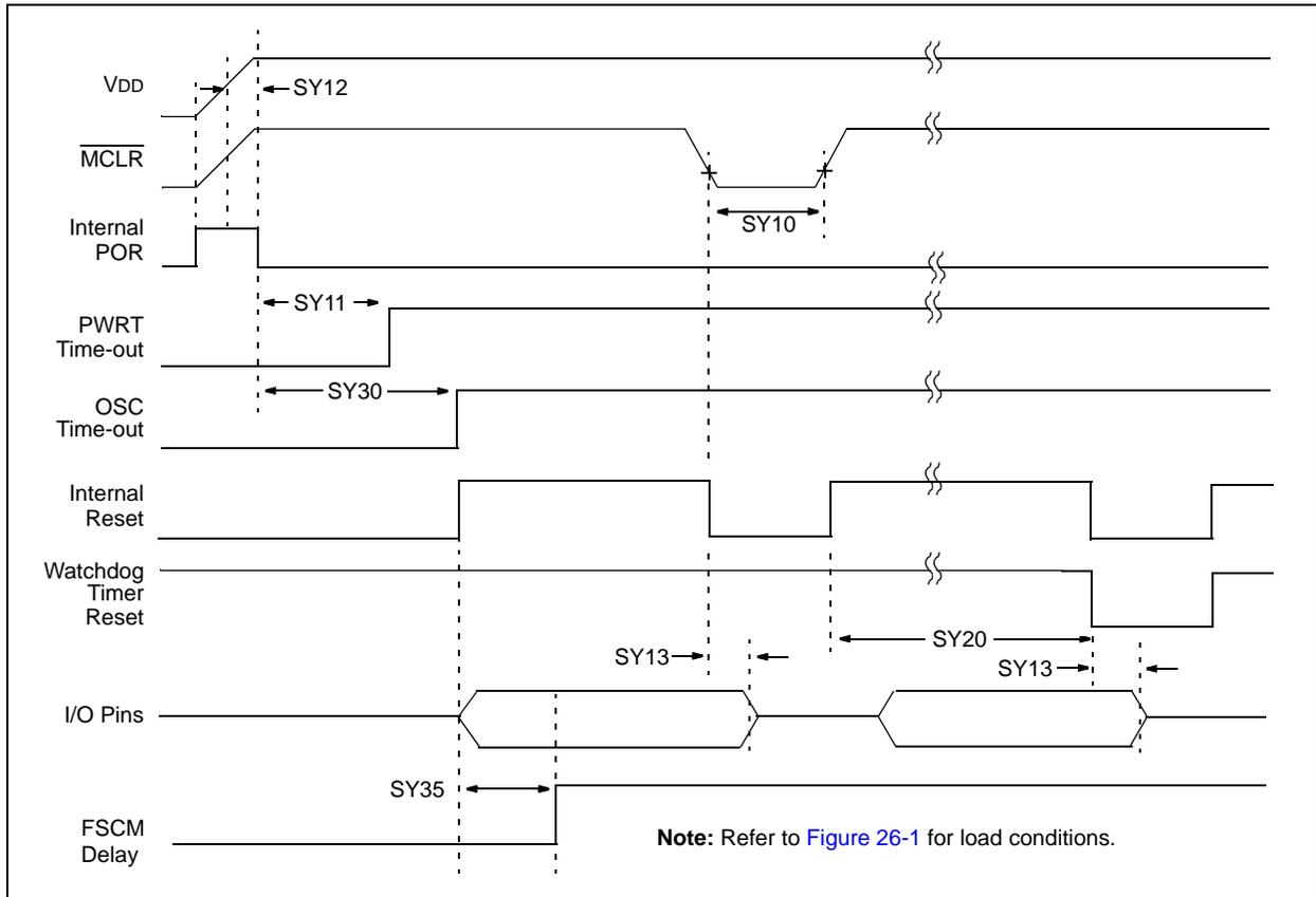
**TABLE 26-21: RESET, WATCHDOG TIMER, OSCILLATOR START-UP TIMER, POWER-UP TIMER TIMING REQUIREMENTS**
